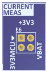
Figure 13. E6 on the Evaluation Kit Board (Top side)
