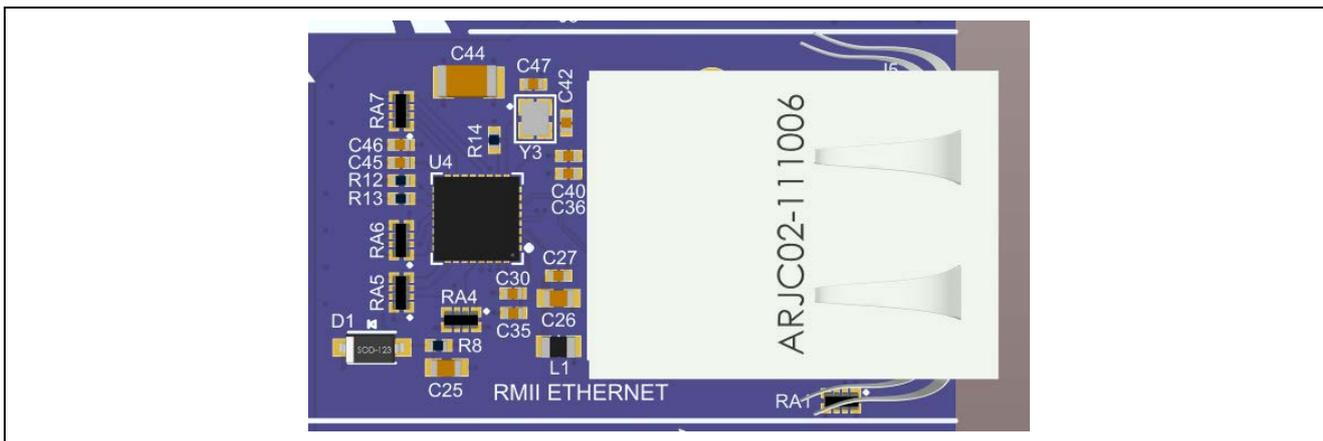
Figure 21. Ethernet Connector
