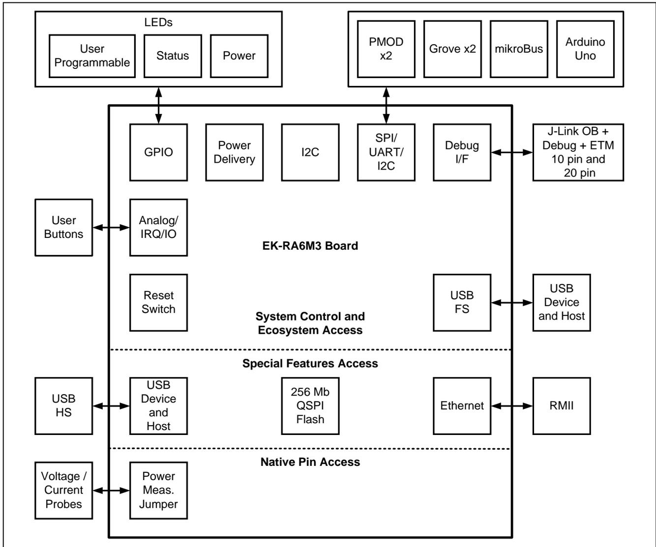
Figure 5. EK-RA6M3 Board Block Diagram
