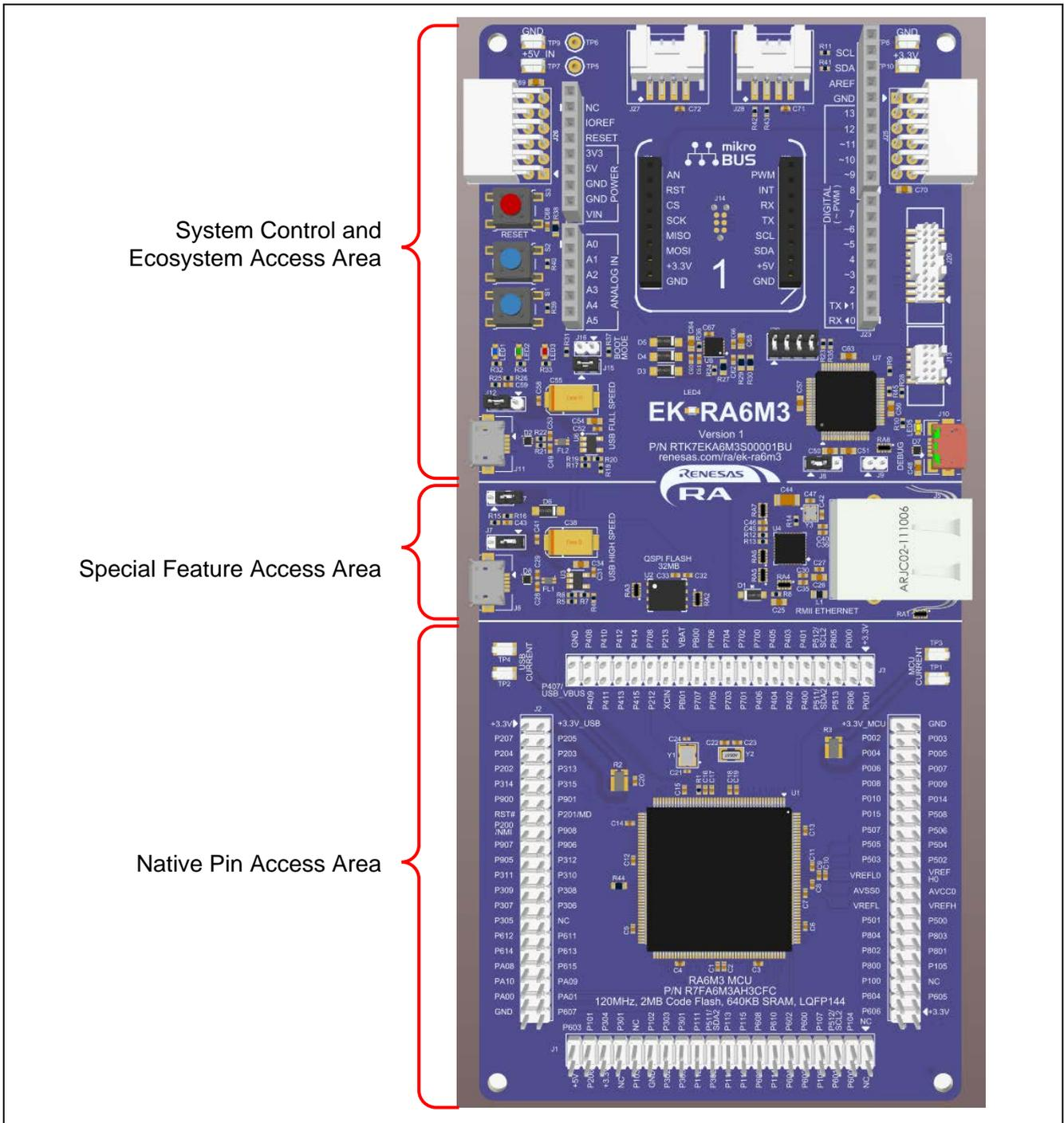
Figure 4. EK-RA6M3 Board Functional Area Definitions
