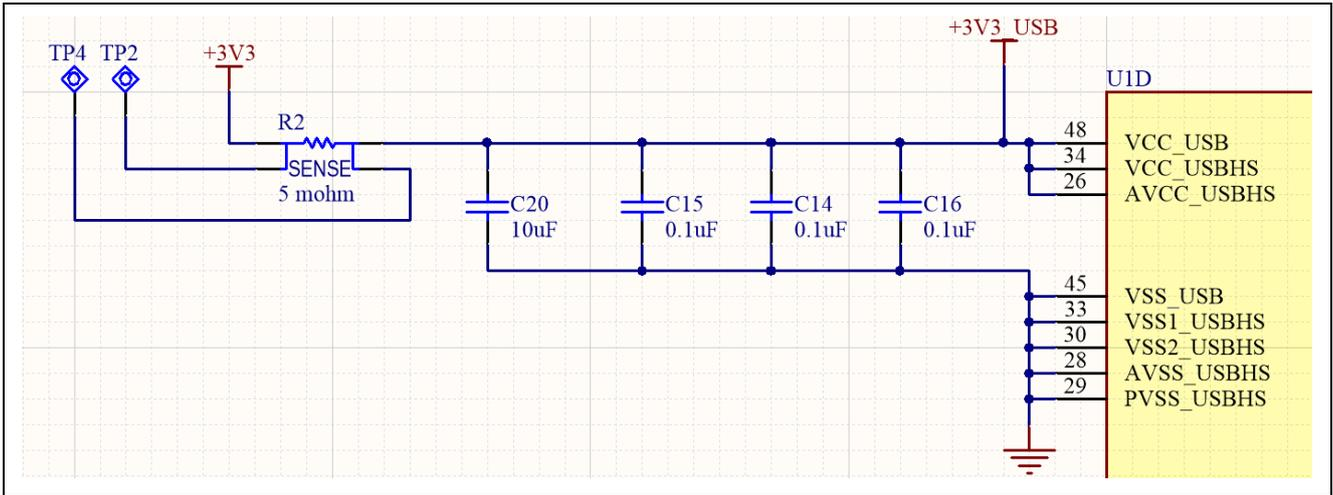
Figure 25. RA USB Current Measurement Circuit
