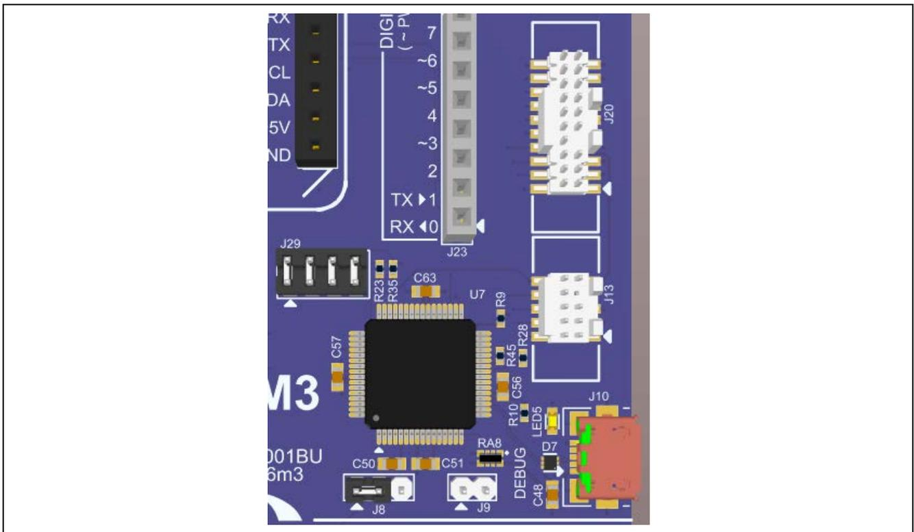
**Figure 9. EK-RA6M3 Debug Interface**
