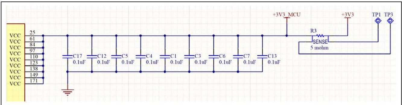
Figure 26. RA +3.3 V Current Measurement Circuit
