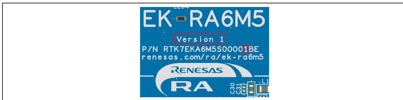
Figure 7. Identification of the Kit Version Number on the EK-RA6M5 Board
