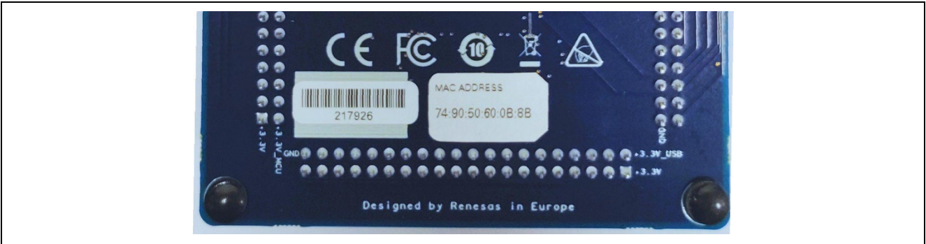
Figure 9. Identification of the Serial Number on the EK-RA6M5 Board
