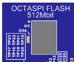
Figure 27. Octo-SPI Flash (labelled as “OCTASPI” on silkscreen text)
