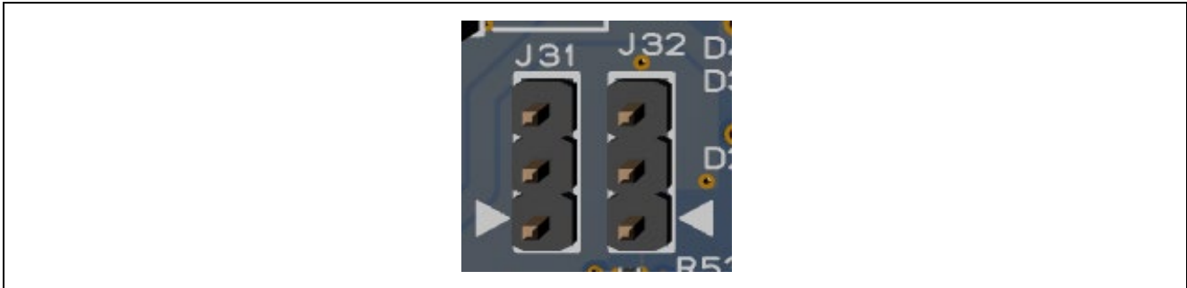
Figure 15. Pmod 1 Pin header jumpers (top side)
