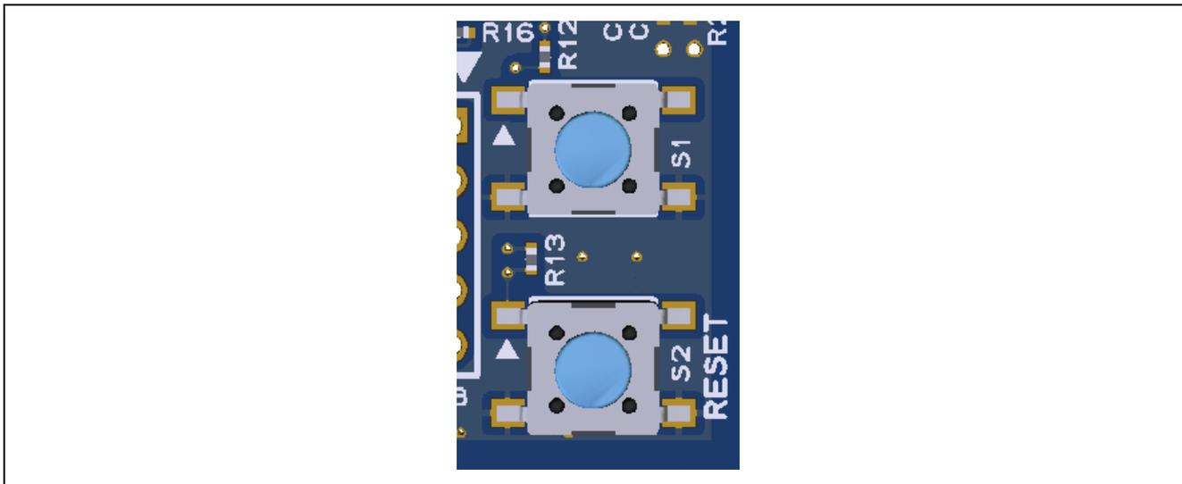
**Figure 21. Reset (S2) and User Switch (S1)**
