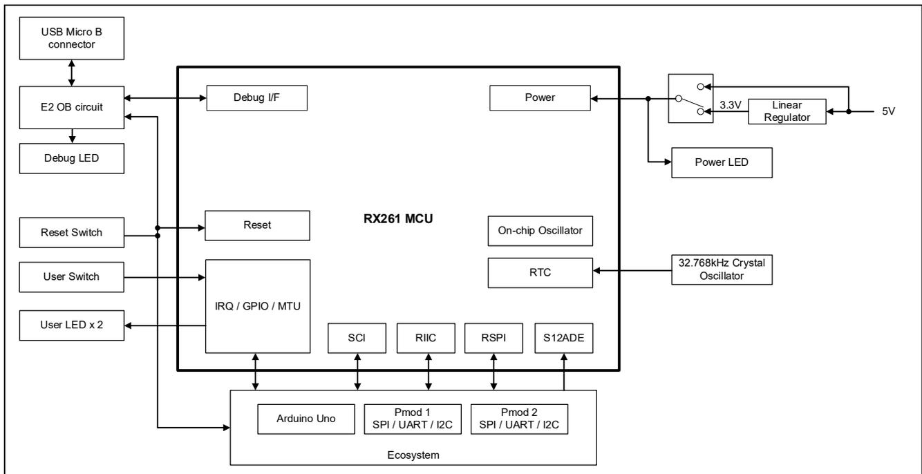
Figure 4. FPB-RX261 v1 Block Diagram
