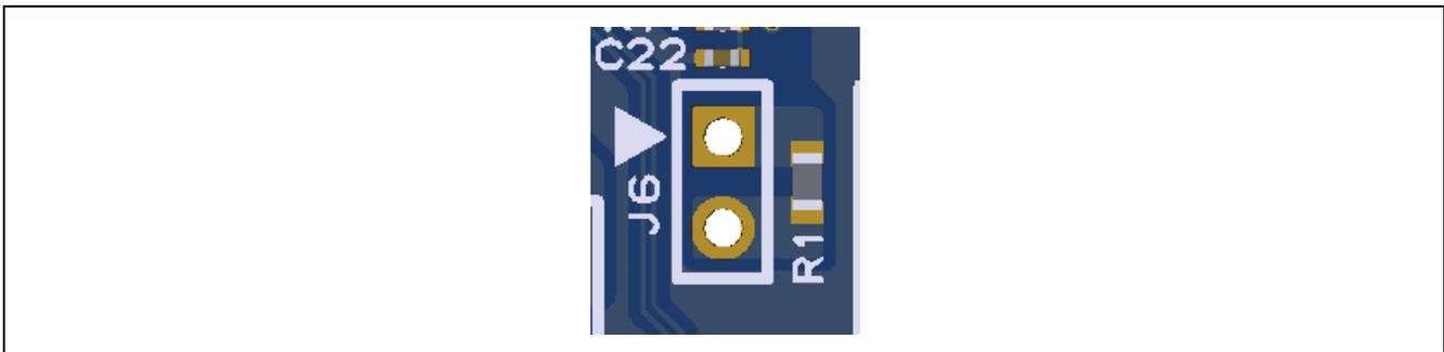
Figure 24. RX MCU Current Measurement Pin Header J6 and R1
