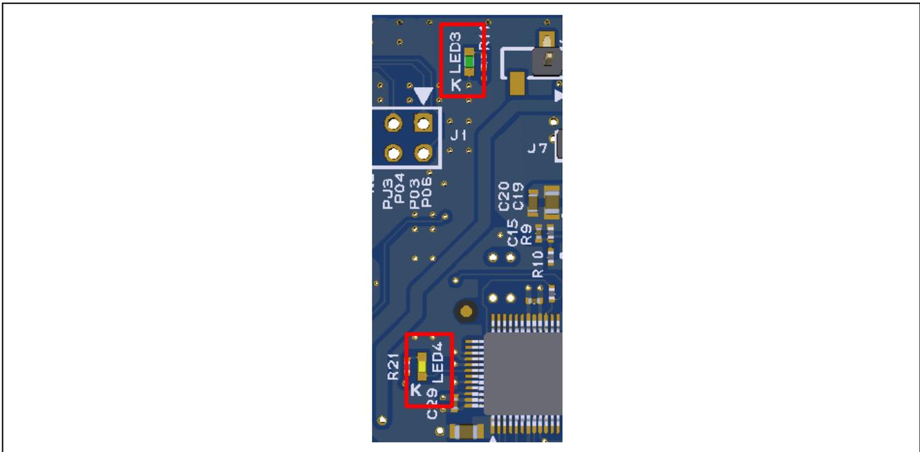
**Figure 20. Power LED and Debug LED**
