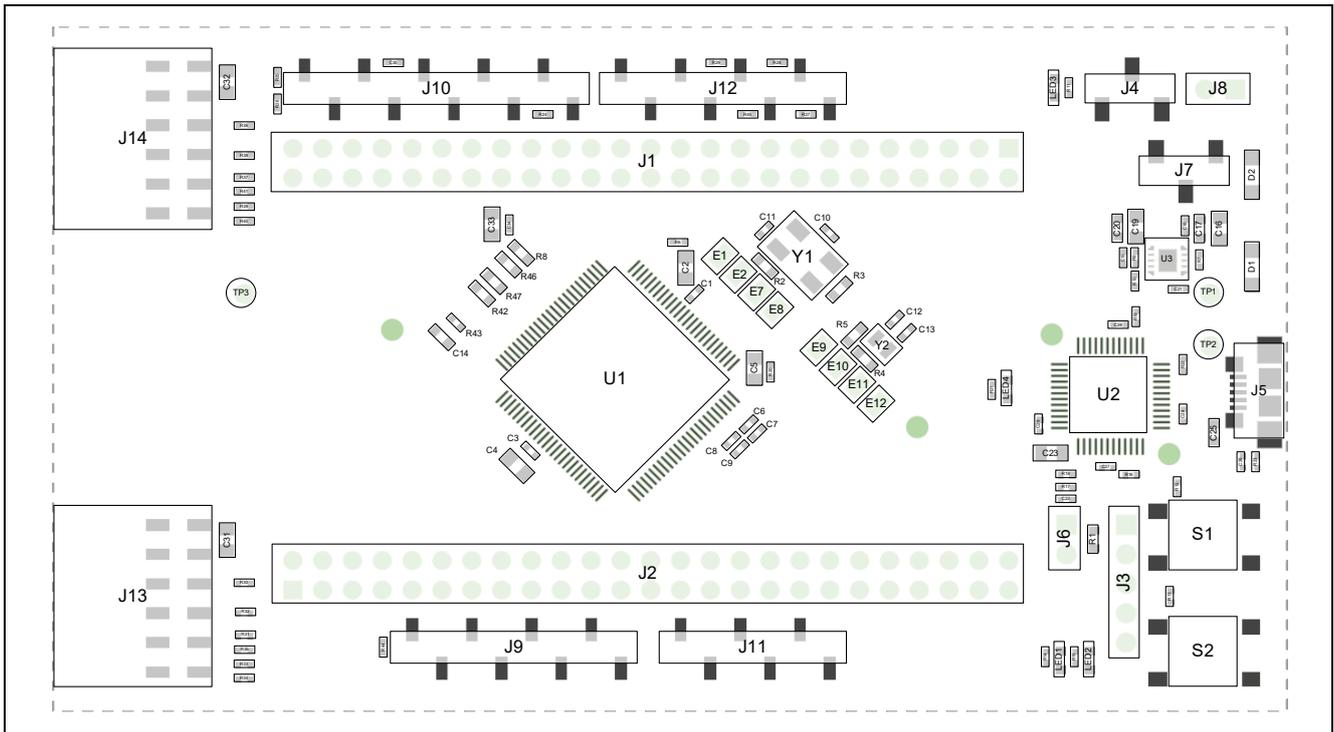
Figure 5. Reference number for components on the FPB-RX261 v1 (top side)
