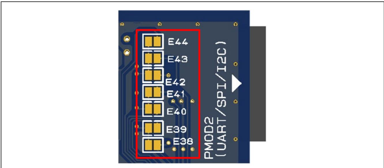
Figure 16. Pmod 2 Copper Jumpers (bottom side)
