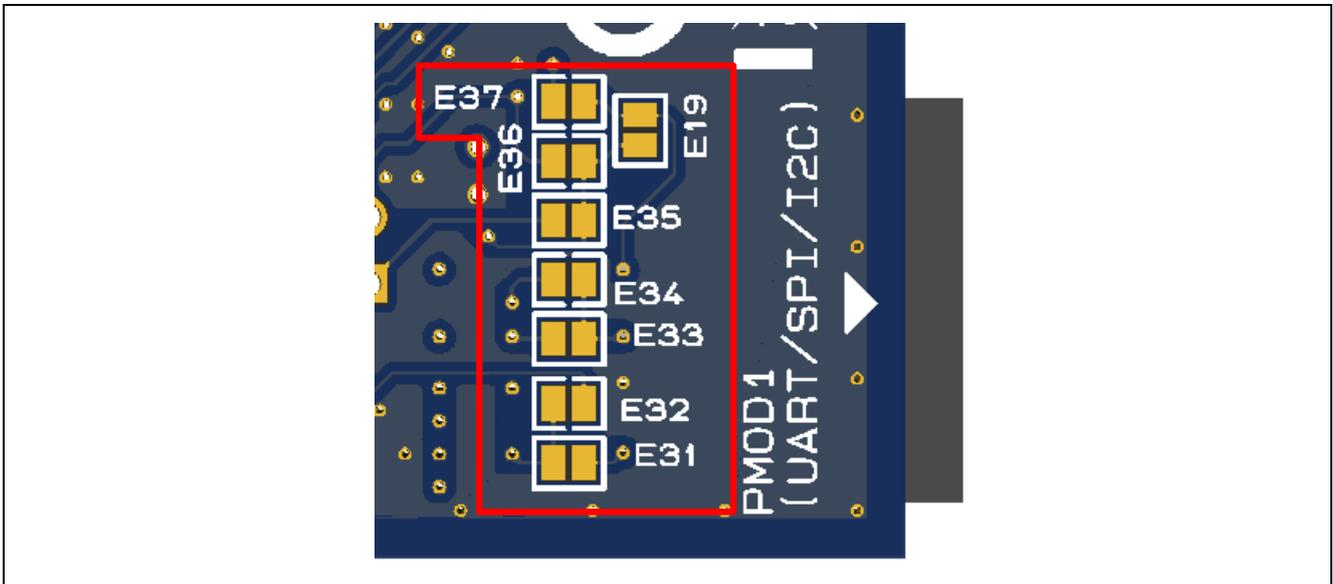
Figure 14. Pmod 1 Copper Jumpers (bottom side)
