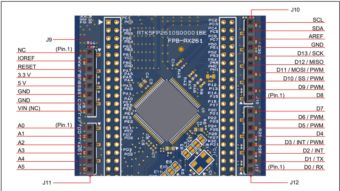
Figure 17. Arduino Uno Connectors
