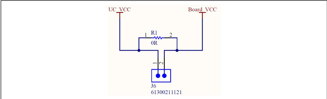
Figure 23. RX MCU Current Measurement Circuit
