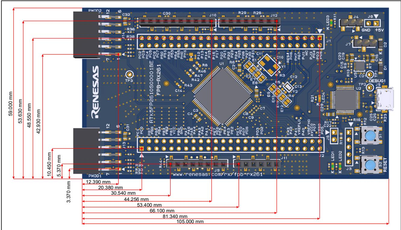
Figure 7. Dimension of the FPB-RX261 v1
