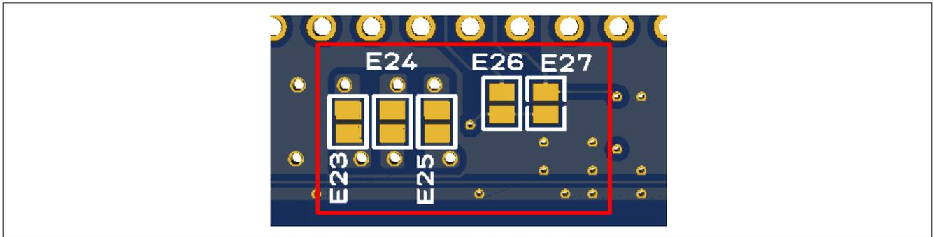
Figure 18. Arduino Uno Copper Jumpers (bottom side)
