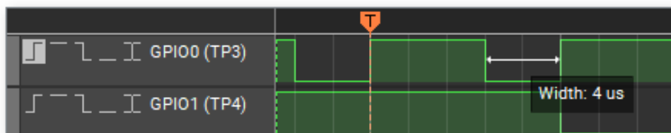
Half Period cursor and sample measurements
