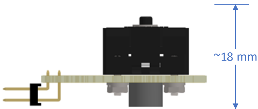
Figure 5. Board Assembly Side View Dimensions
