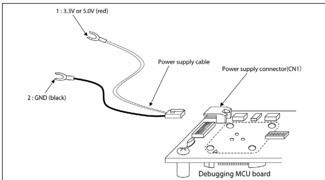
**Figure 5.2 Connection of the Power Supply Connector**
