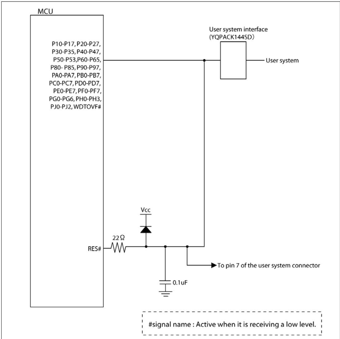
Figure 6.1 Wiring on the Debugging MCU Board (1)
