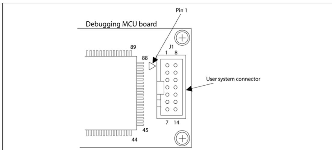
**Figure 5.1 Top View of the User System Connector**
