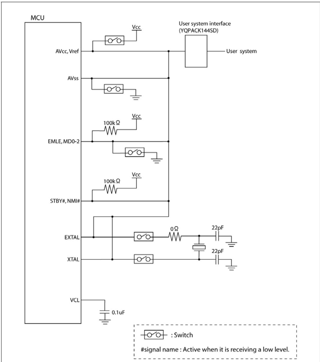
Figure 6.2 Wiring on the Debugging MCU Board (2)
