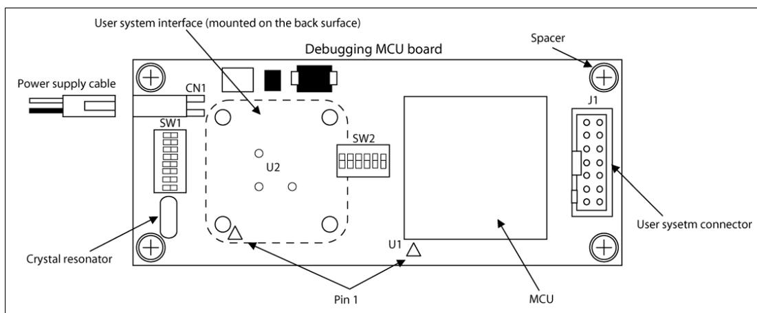
**Figure 1.1 External Appearance of the Debugging MCU Board**
