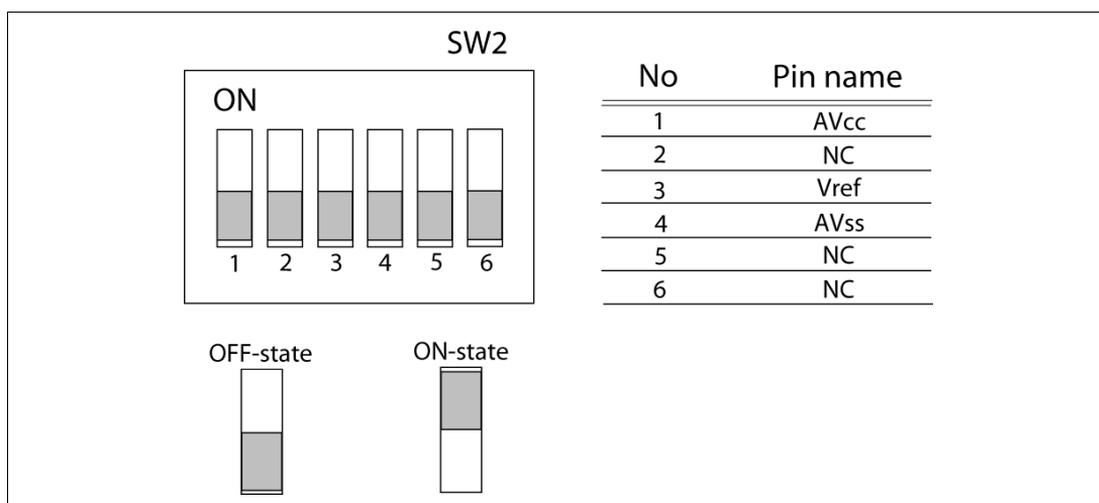
**Figure 4.3 Allocation to the Power Switches**
