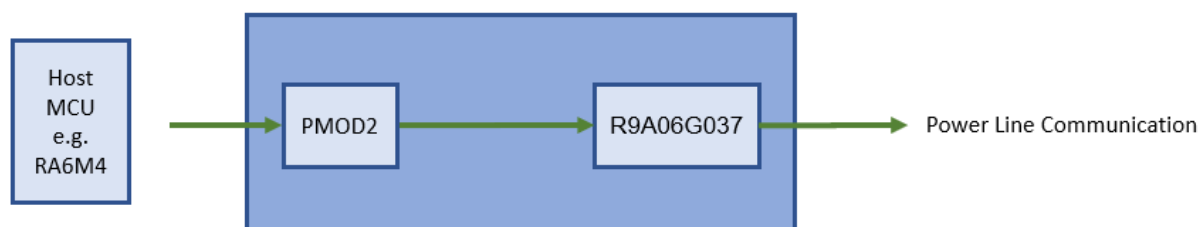
Figure 24: PMOD2 to R9A06G037 Connection (PLC Only) Block Diagram.
