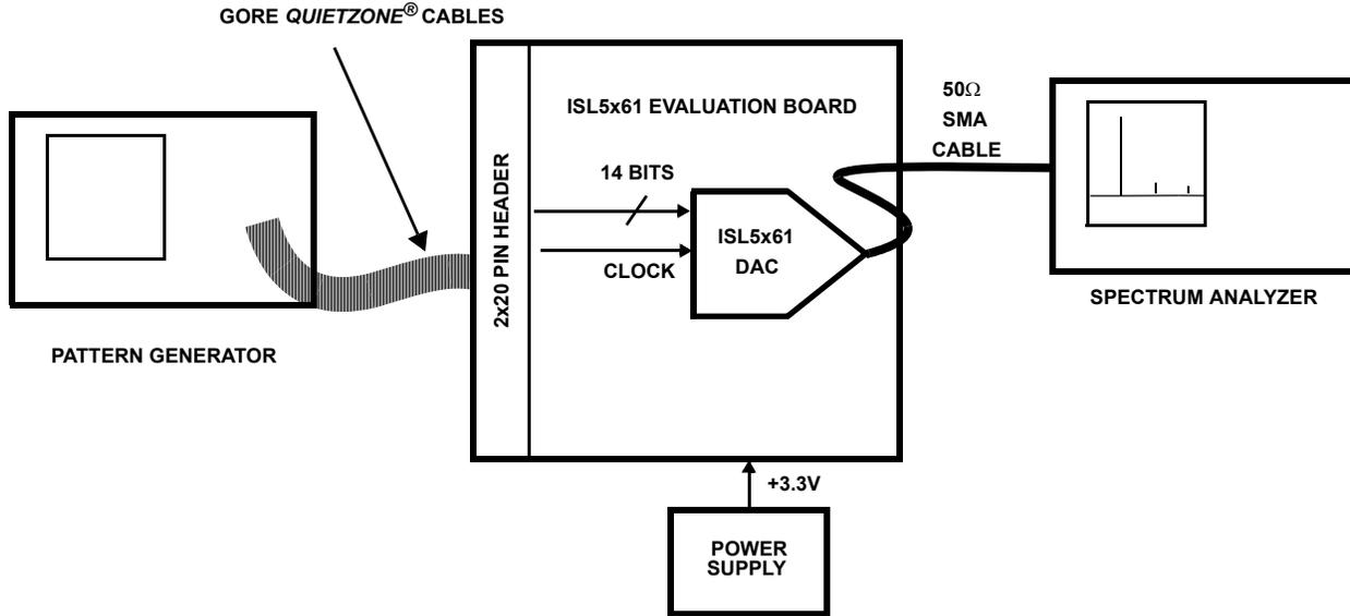
FIGURE 1. INTERSIL ISL5x61 EVALUATION SYSTEM SETUP BLOCK DIAGRAM
