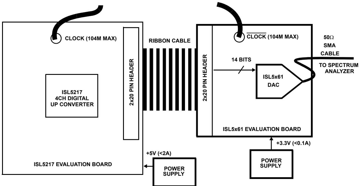
FIGURE 2. INTERSIL ISL5x61 + ISL5217 SETUP BLOCK DIAGRAM
