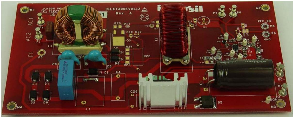
FIGURE 2. TOP VIEW OF THE EVALUATION BOARD
