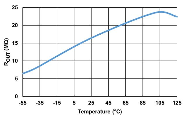
Figure 13. Output Impedance (R<sub>OUT</sub>) vs Temperature
