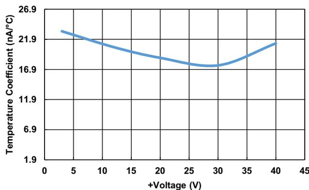
Figure 12. Output Current Temperature Coefficient vs Voltage
