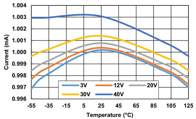
Figure 9. Output Current vs Temperature vs Voltage
