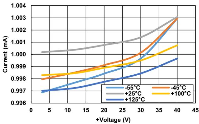
Figure 8. Output Current vs Voltage vs Temperature
