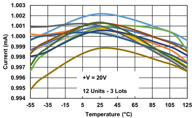
Figure 10. Output Current vs Temperature vs (12 units - 3 lots)
