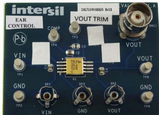
FIGURE 1. VOLTAGE REFERENCE EVALUATION BOARD
