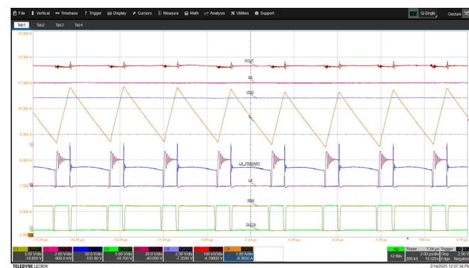
Figure 34. Waveforms with VIN 28V and 10A Load
