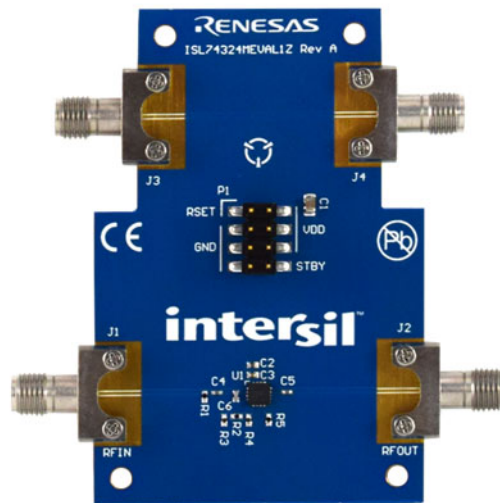
Figure 2. ISL74324MEVAL1Z Evaluation Board (Top)
