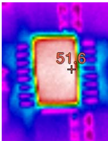
Figure 11. Case Temperature V_H = V_{S+} = 15V , 1MHz, 4 Channels, T_A = +25^\circ C
