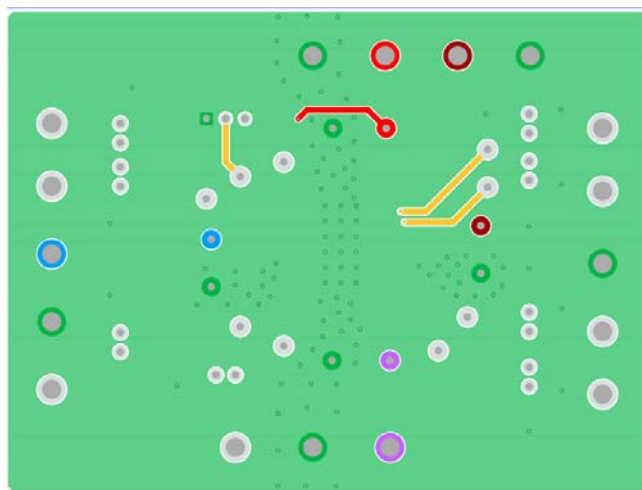
Figure 7. Bottom Trace Layer
