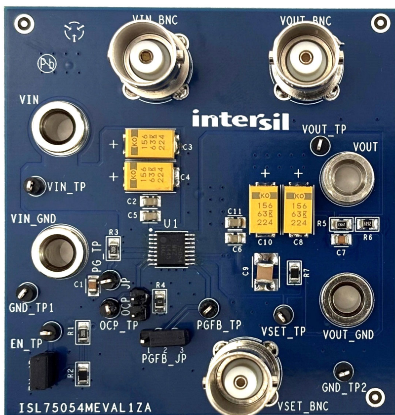
Figure 2. ISL75054MEVAL1Z Evaluation Board (Top)
