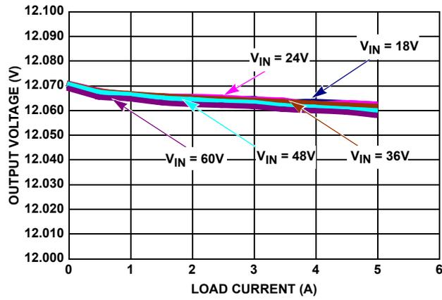
FIGURE 9. LINE REGULATION FOR V<sub>OUT</sub> = 12V
