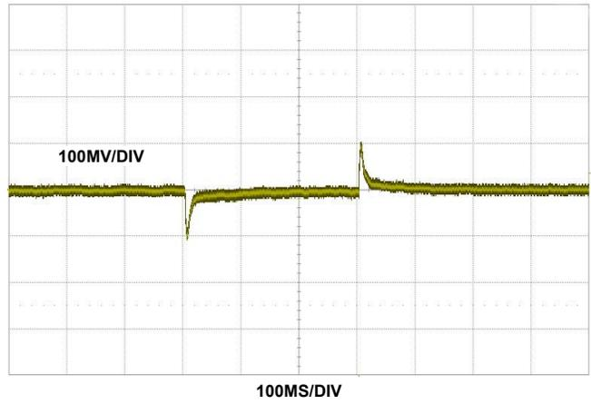
FIGURE 12. 1V<sub>OUT</sub> TRANSIENT RESPONSE, I<sub>OUT</sub> = 0A TO 20A, f<sub>SW</sub> = 350kHz, LOAD CURRENT SLEW RATE: 10A/μs
