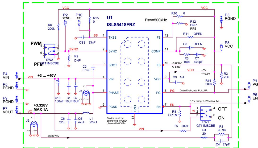
FIGURE 10. ISL85418EVAL1Z SCHEMATIC
