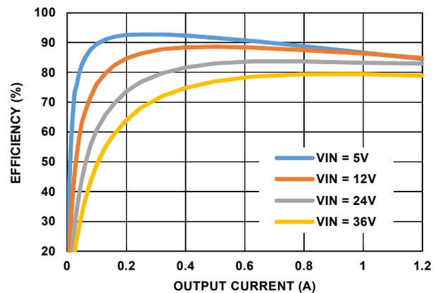
FIGURE 20. EFFICIENCY, PWM (ISL854102EVAL1Z,  $V_{OUT} = 3.3V$ )
