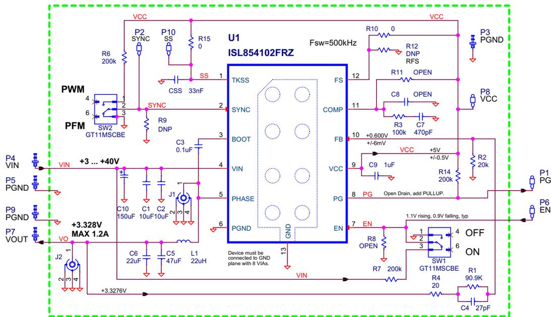
FIGURE 9. ISL854102EVAL1Z SCHEMATIC
