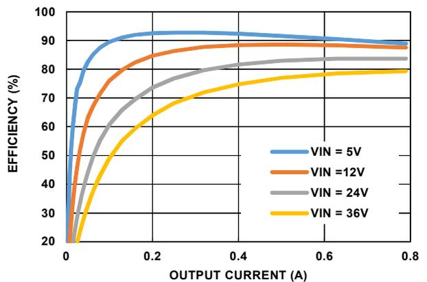
FIGURE 22. EFFICIENCY, PWM (ISL85418EVAL1Z,  $V_{OUT} = 3.3V$ )
