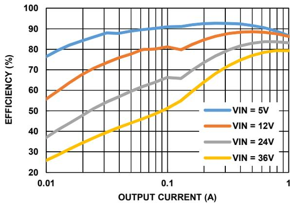
FIGURE 17. EFFICIENCY, PFM (ISL85410EVAL1Z,  $V_{OUT} = 3.3V$ )
