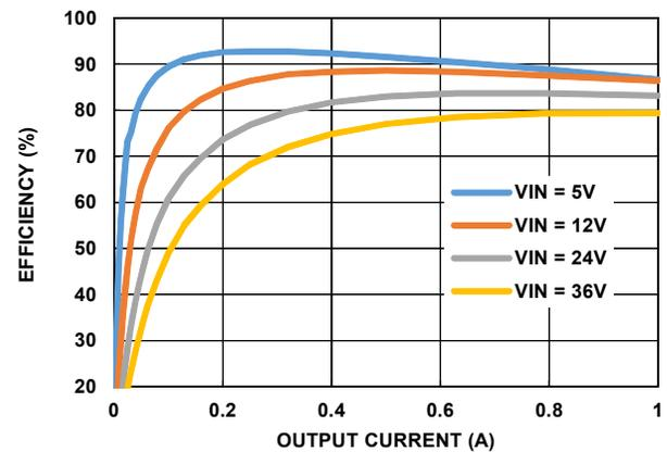
FIGURE 18. EFFICIENCY, PWM (ISL85410EVAL1Z,  $V_{OUT} = 3.3V$ )
