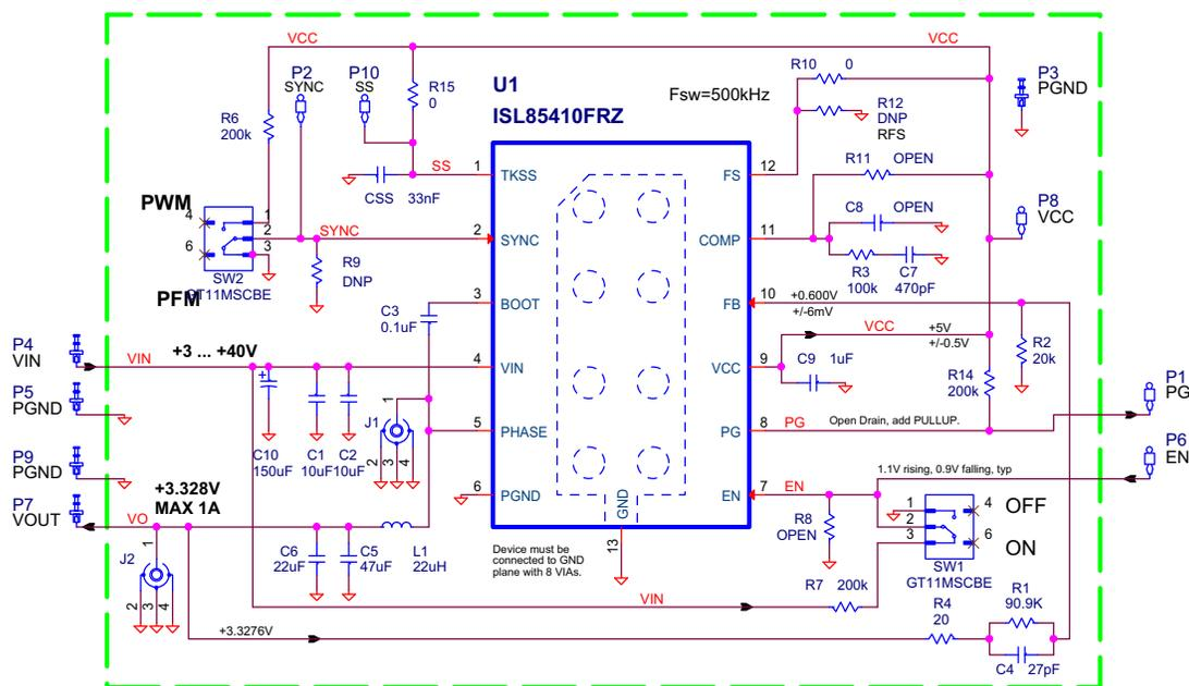
FIGURE 8. ISL85410EVAL1Z SCHEMATIC
