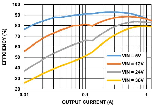
FIGURE 19. EFFICIENCY, PFM (ISL854102EVAL1Z,  $V_{OUT} = 3.3V$ )
