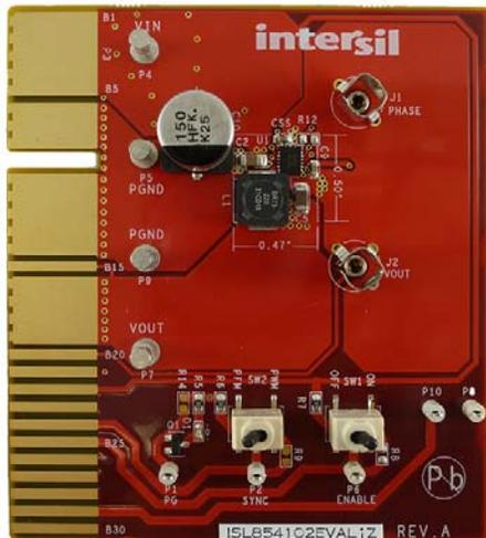
FIGURE 4. FRONT OF EVALUATION BOARD ISL854102EVAL1Z
