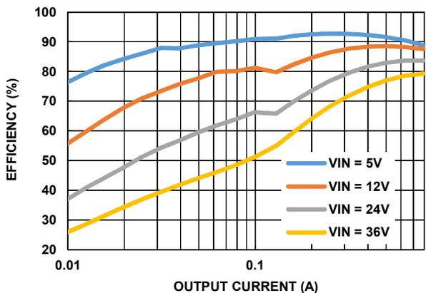
FIGURE 21. EFFICIENCY, PFM (ISL85418EVAL1Z,  $V_{OUT} = 3.3V$ )
