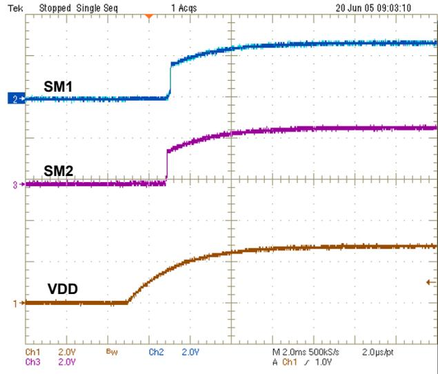
FIGURE 3. TYPICAL SM1 AND SM2 TURN ON
