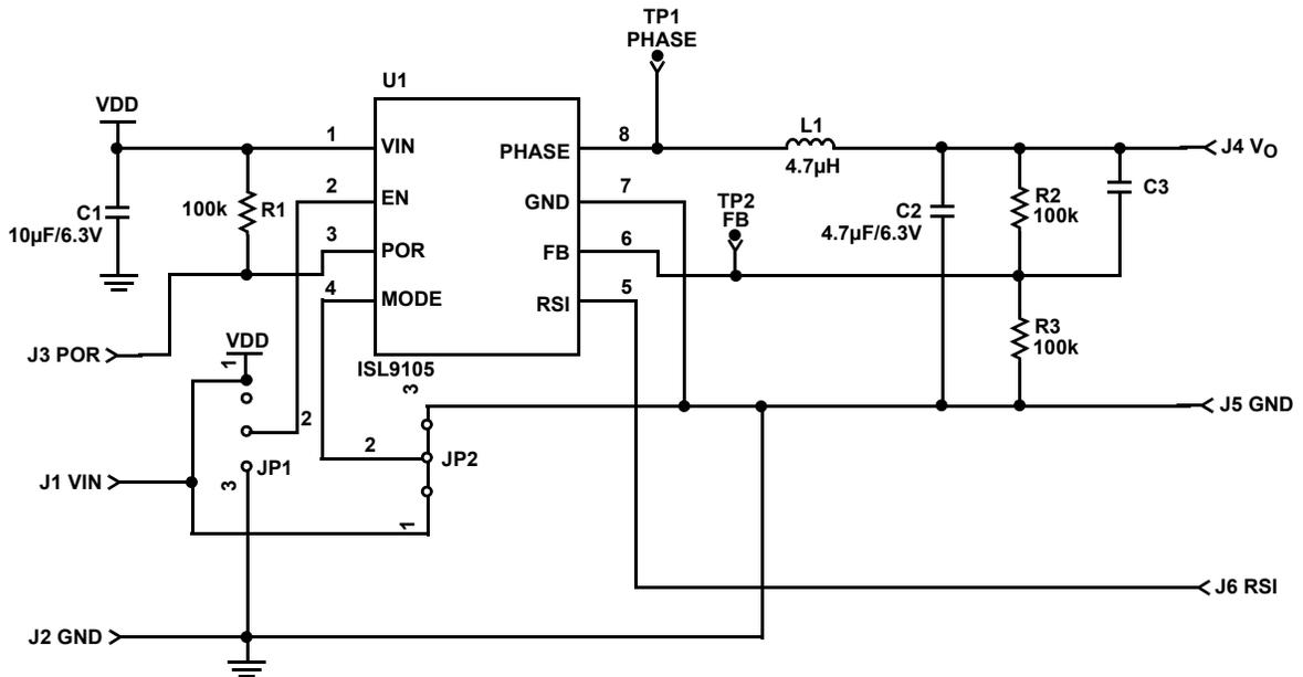
FIGURE 2. ISL9105EVAL1Z SCHEMATIC
