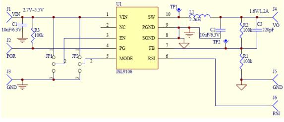
FIGURE 1. ISL9106EVAL1Z SCHEMATIC
