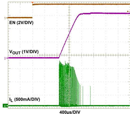
FIGURE 3. SOFT-START ( $V_{IN} = 4\text{V}$ ,  $V_{OUT} = 3.3\text{V}$ , NO LOAD)
