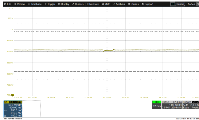
Figure 60. VDDIO_VTO Output Voltage Transient Response, ISL75055, (VDDIO_x (Complex)/2)±1A, ±90mV Limits, VDDIO_x (Complex) = 1.8V
