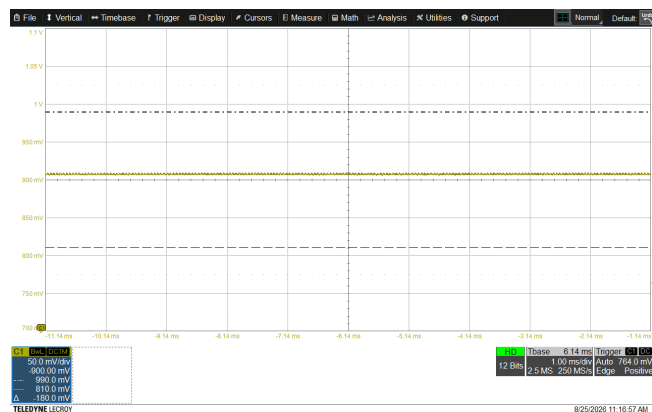
Figure 36. VDDIO_VTO Output Voltage, ISL75055, (VDDIO_x (Complex)/2)/±1A, ±90mV Limits, VDDIO_x (Complex) = 1.8V
