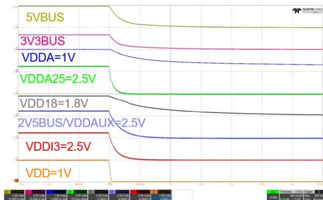
Figure 40. Shutdown, Rails 1-8, 50mA on VDD
