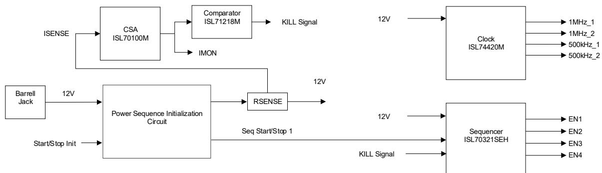
**Figure 3. Renesas Radiation Tolerant Power Tree for Microchip RT PolarFire FPGA**
