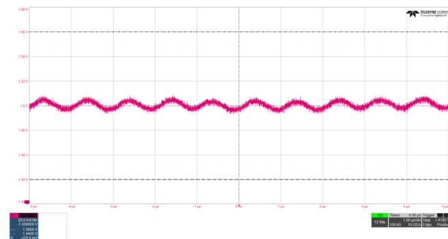
**Figure 18. VDDI[2,4,5] Output Voltage Ripple, ISL73007,
