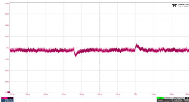
**Figure 31. VDDI[0,1,6,7] Output Voltage, Load Transient Response, ISL73007, 1.2V at 25% to 75% Load Step,  $\pm 120\text{mV}$  Limits**
