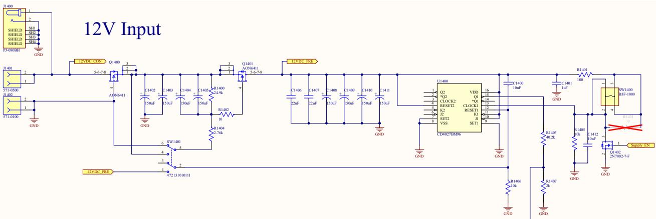
Figure 9. 12V Input and Sequencer Initialization
