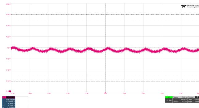
**Figure 17. VDDI[0,1,6,7] Output Voltage Ripple,
