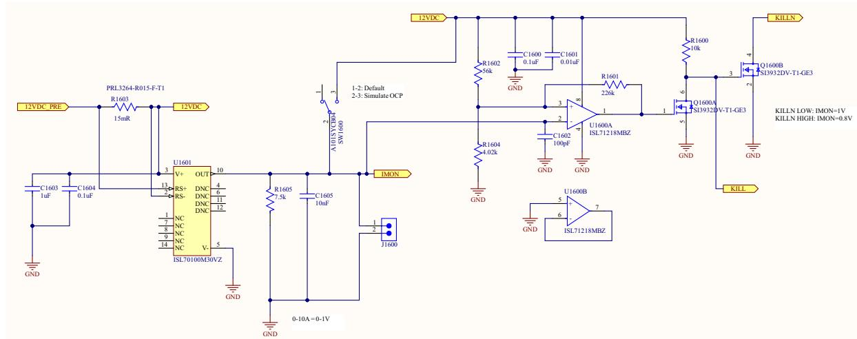
**Figure 11. ISL70100 Input Current Sense Schematic**
