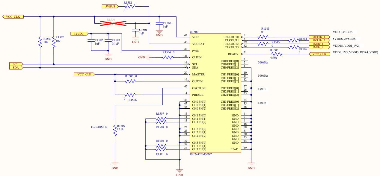
Figure 10. ISL74420 Quad Clock Schematic
