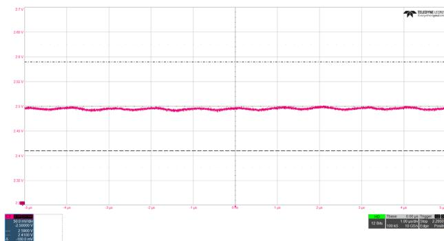
**Figure 19. VDDI3 Output Voltage Ripple, ISL73007,
