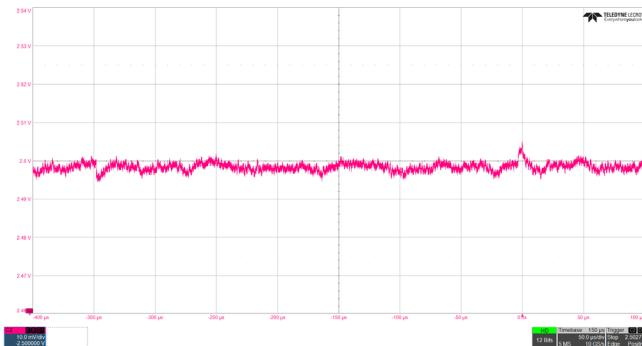
**Figure 29. VDD25/VDDA25 Output Voltage, Load Transient Response, ISL75054, 2.5V at 25% to 75% Load Step,  $\pm 200\text{mV}$  Limits**
