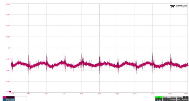
**Figure 26. 5VBUS Output Voltage Ripple, ISL73007, 5V/2A**
