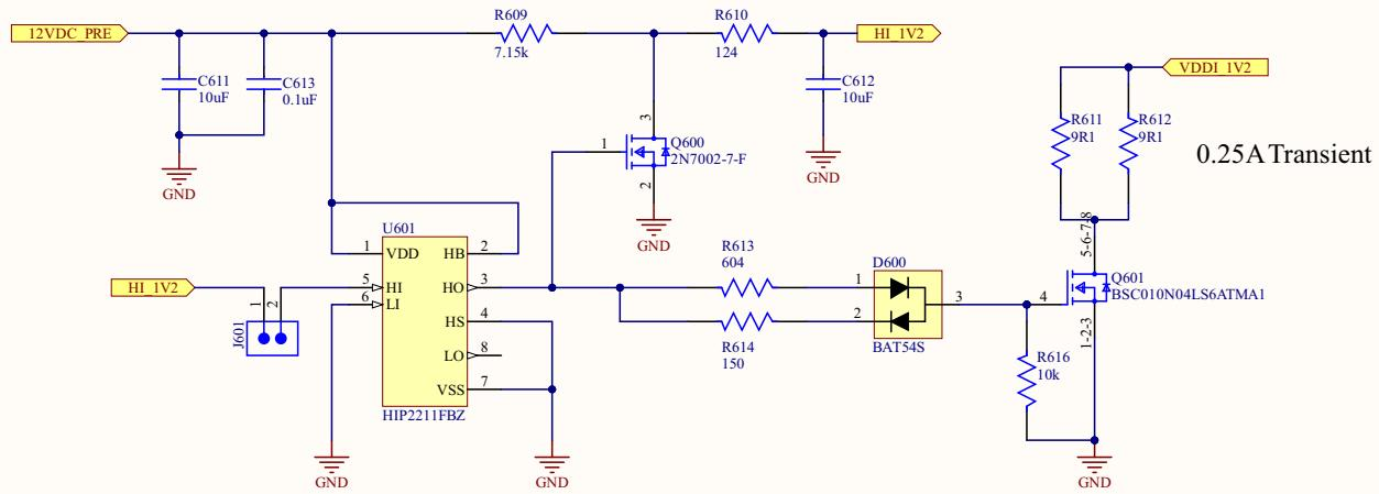
Figure 6. Typical Load Transient Circuit using HIP2211 HB Driver
