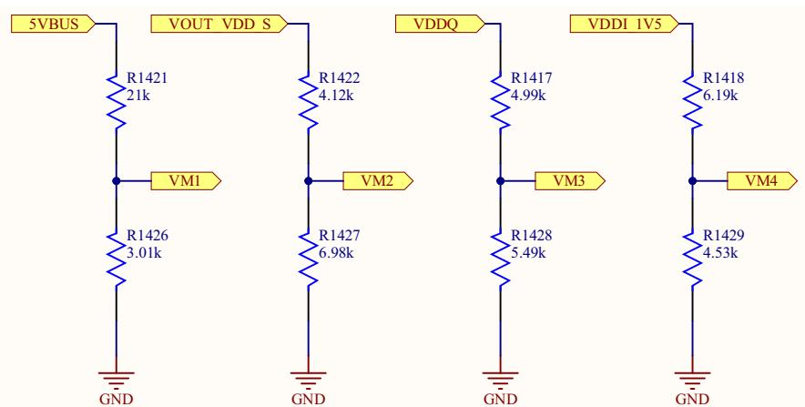
Figure 8. Power Supply Sequence Voltage Monitor Dividers
