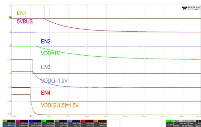
Figure 42. Sequencer Shutdown, 50mA Load (All Four Rails)
