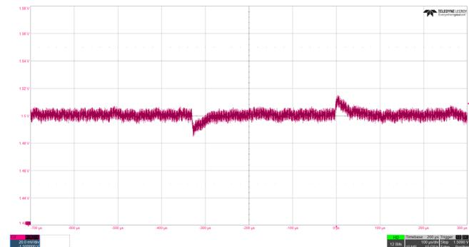
**Figure 32. VDDI[2,4,5] Output Voltage, Load Transient Response, ISL73007, 1.5V at 25% to 75% Load Step,  $\pm 150\text{mV}$  Limits**
