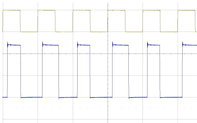
Figure 52. 5VBUS Switching Waveform, ISL73007, 5V/2A, (C1 = SYNC, C3 = LX)
