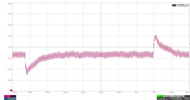
**Figure 34. VDDAUX[2,4,5]/VPP/2V5BUS Output Voltage, Load Transient Response, ISL73007, 2.5V at 25% to 75% Load Step,  $\pm 200\text{mV}$  Limits**
