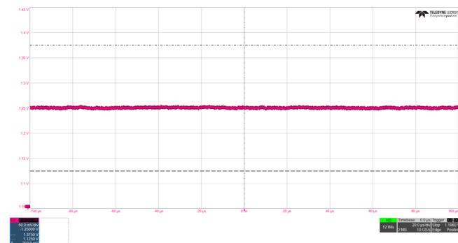
**Figure 22. XCVR\_VREF Output Voltage, 3A Source/Sink
