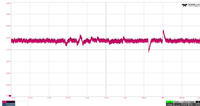
**Figure 35. 3V3BUS Output Voltage, Load Transient Response, ISL73007, 3.3V w/ Downstream Transient Generators Enabled (VDDA, VDD25, VDD18, VDDI[0,1,6,7], VDDI[2,4,5], VDDI3)**
