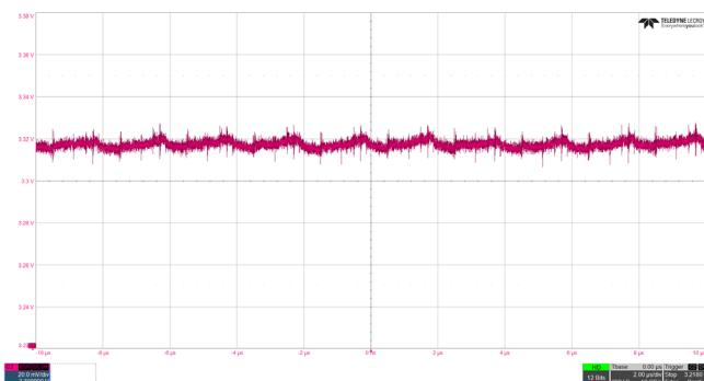
**Figure 25. 3V3BUS Output Voltage Ripple, ISL73007, 3.3V/3A**
