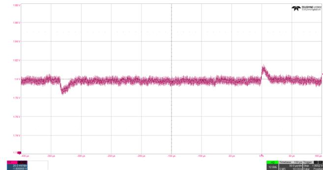
**Figure 30. VDD18 Output Voltage, Load Transient Response, ISL73007, 1.8V at 25% to 75% Load Step,  $\pm 200\text{mV}$  Limits**
