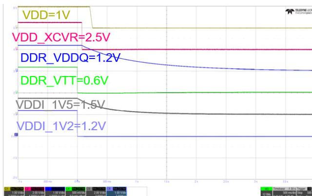
Figure 39. Shutdown, Rails 8 to 13, 50mA on VDD, VDDI\_1V2
