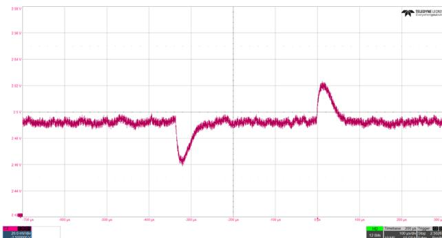
**Figure 33. VDDI3 Output Voltage, Load Transient Response, ISL73007, 2.5V at 25% to 75% Load Step,  $\pm 180\text{mV}$  Limits**
