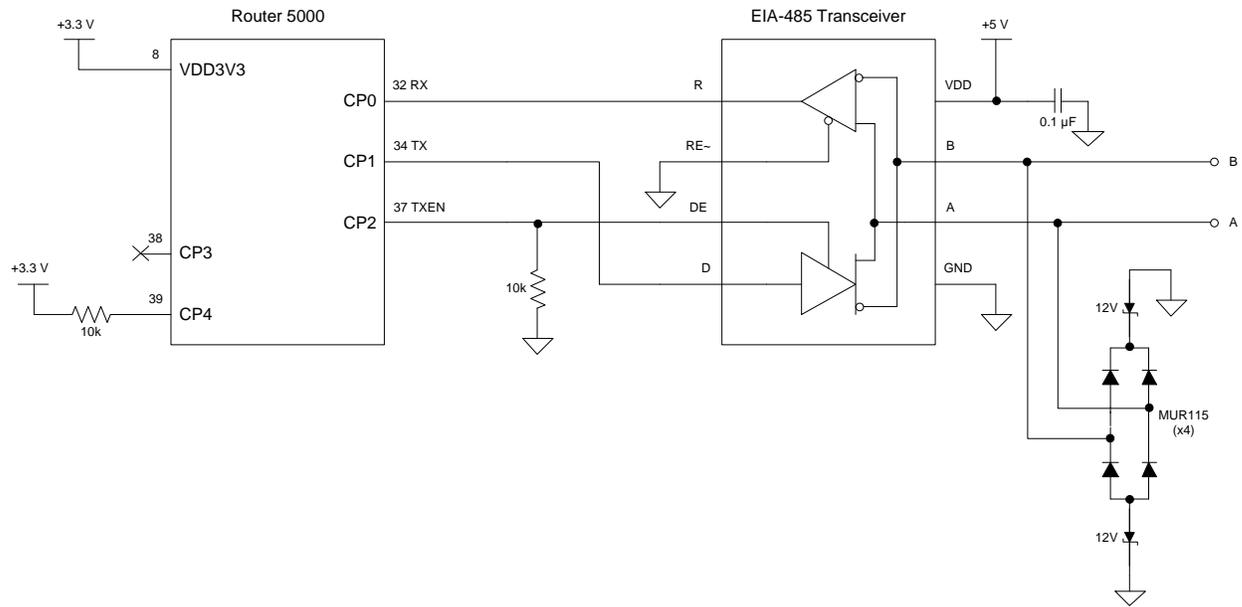
**Figure 33.** EIA-485 Twisted-Pair Interface (Uses Single-Ended Mode)
