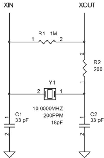
**Figure 13.** Series 5000 Chip Clock Generator Circuit
