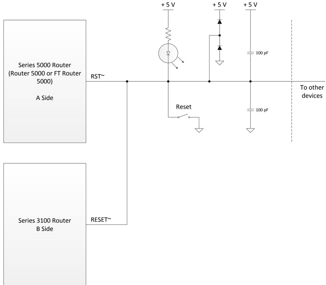
**Figure 17.** Reset Circuit – Series 5000 Router with Series 3100 Router
