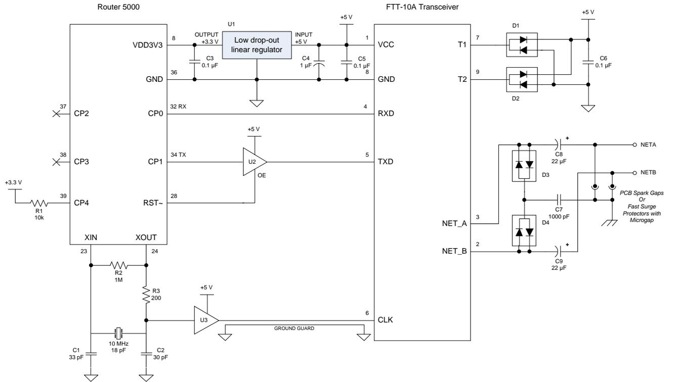
**Figure 34.** Connecting a Router 5000 to an FTT-10A Transceiver
