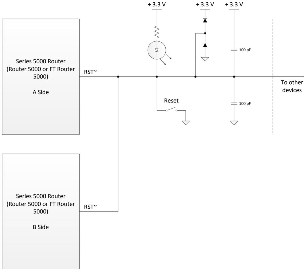
**Figure 16.** Reset Circuit – Series 5000 Router for Both Halves
