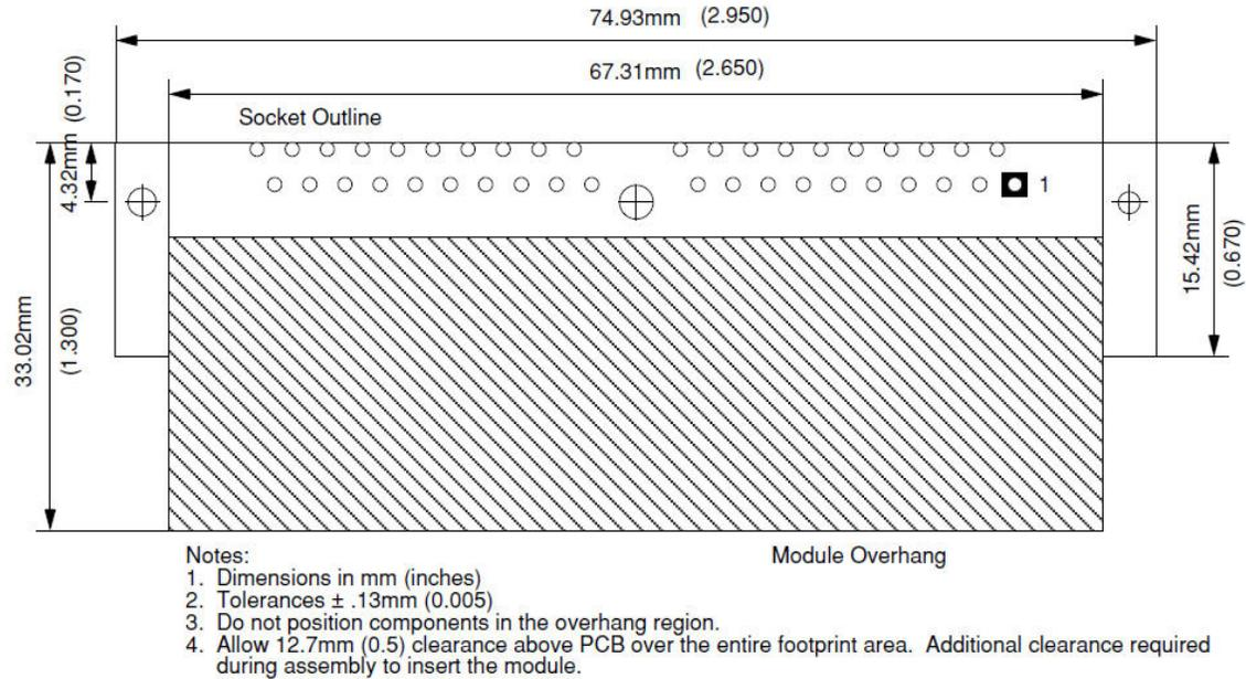
**Figure 24.** RTR-10 PCB Footprint (Component Side, Horizontal Mounting)
