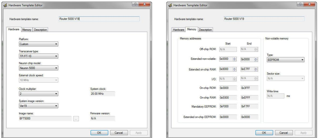
**Figure 40.** Example NodeBuilder Hardware Template for the Router 5000
