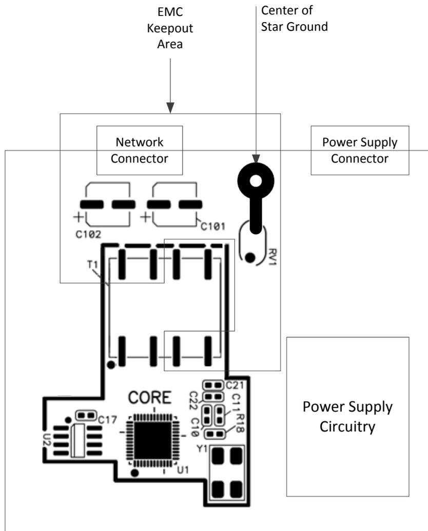
**Figure 43.** Example PCB Layout for an FT Router 5000
