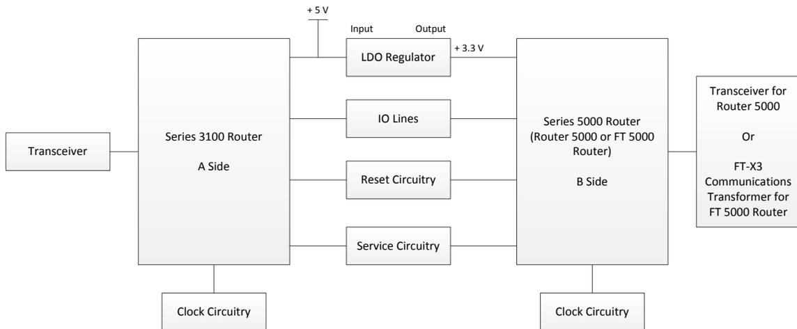
**Figure 39.** Basic Connections for Series 3100 and Series 5000 Half-Routers
