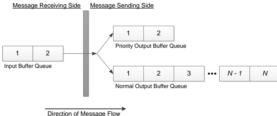
**Figure 8.** Buffering Scheme for a LONWORKS Router
