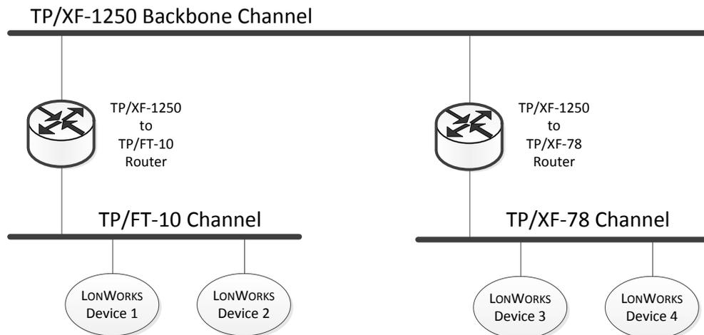
**Figure 1.** Sample Router Installation
