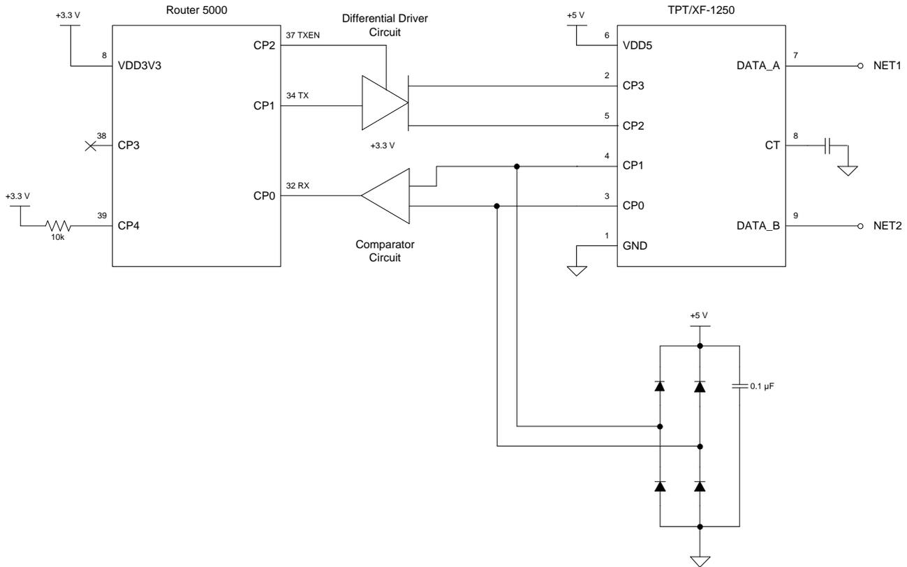
**Figure 30.** Connecting a Router 5000 to a TP/XF-1250 Transceiver
