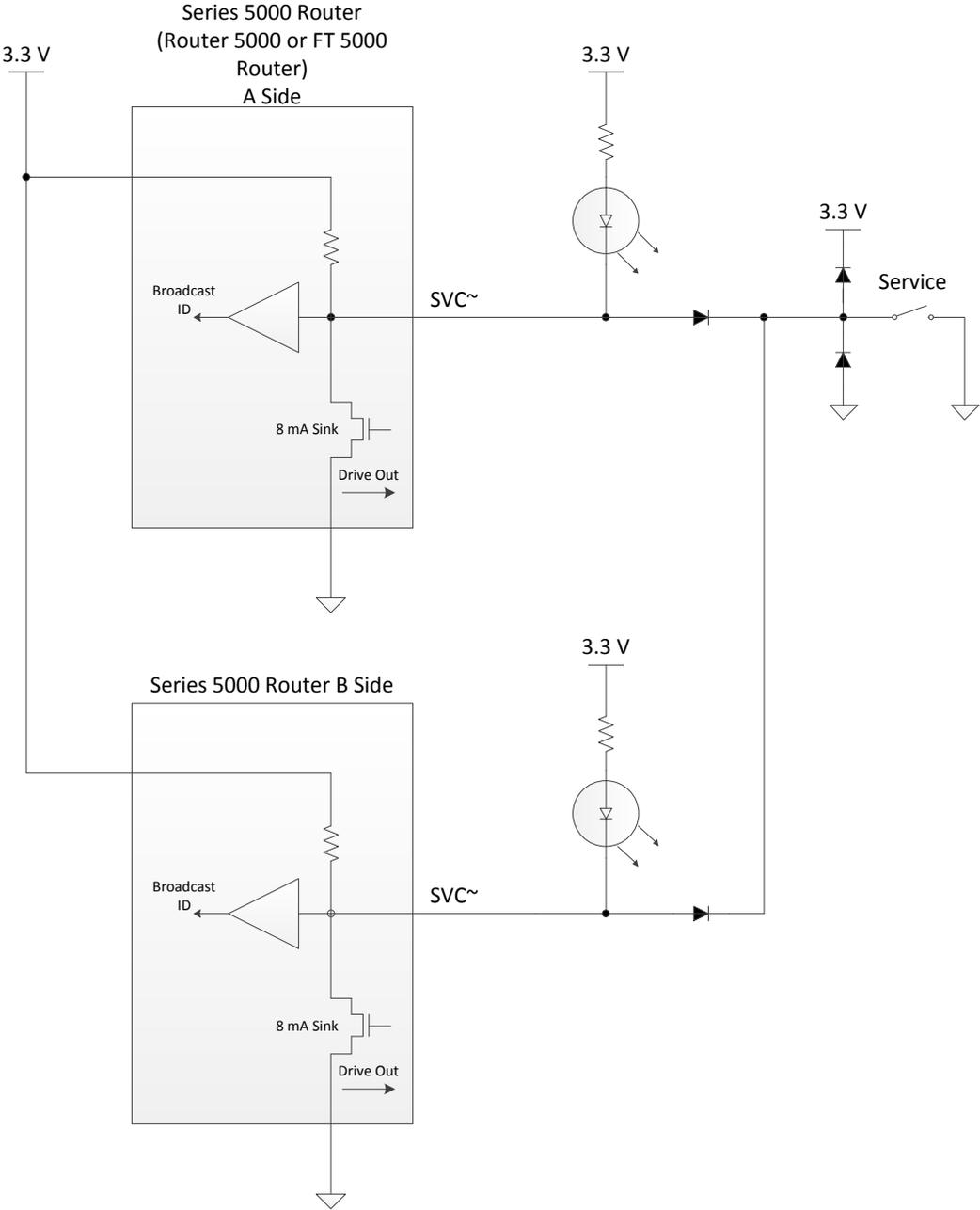
**Figure 18.** Service Circuit – Series 5000 Router for Both Halves
