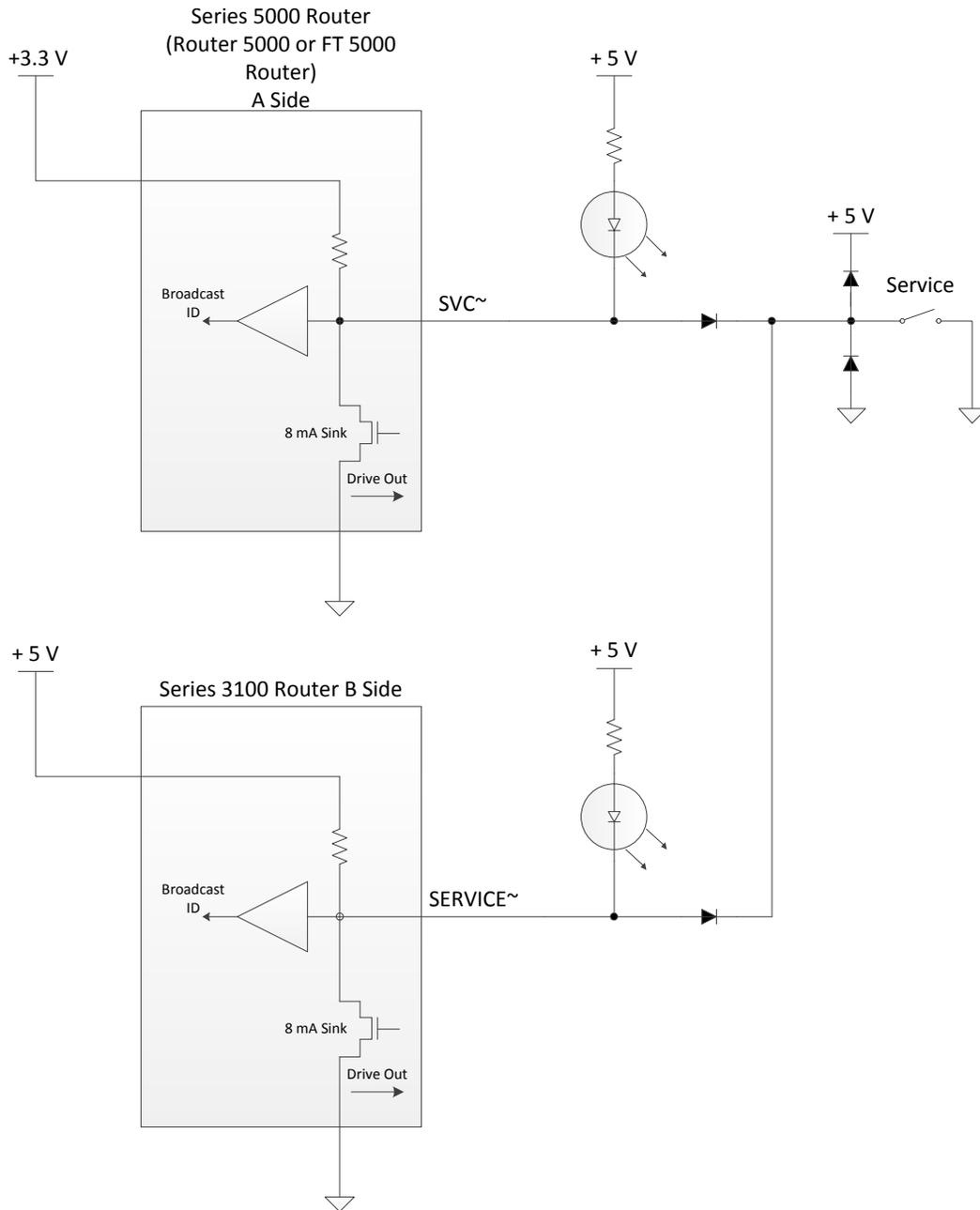
**Figure 19.** Service Circuit – Series 5000 Router with Series 3100 Router
