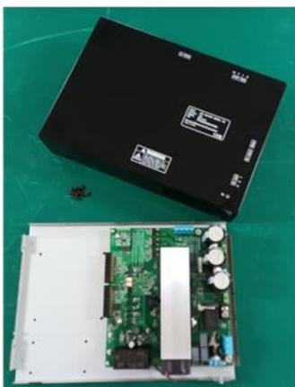
Fig. 3-1 Removing the main body cover
