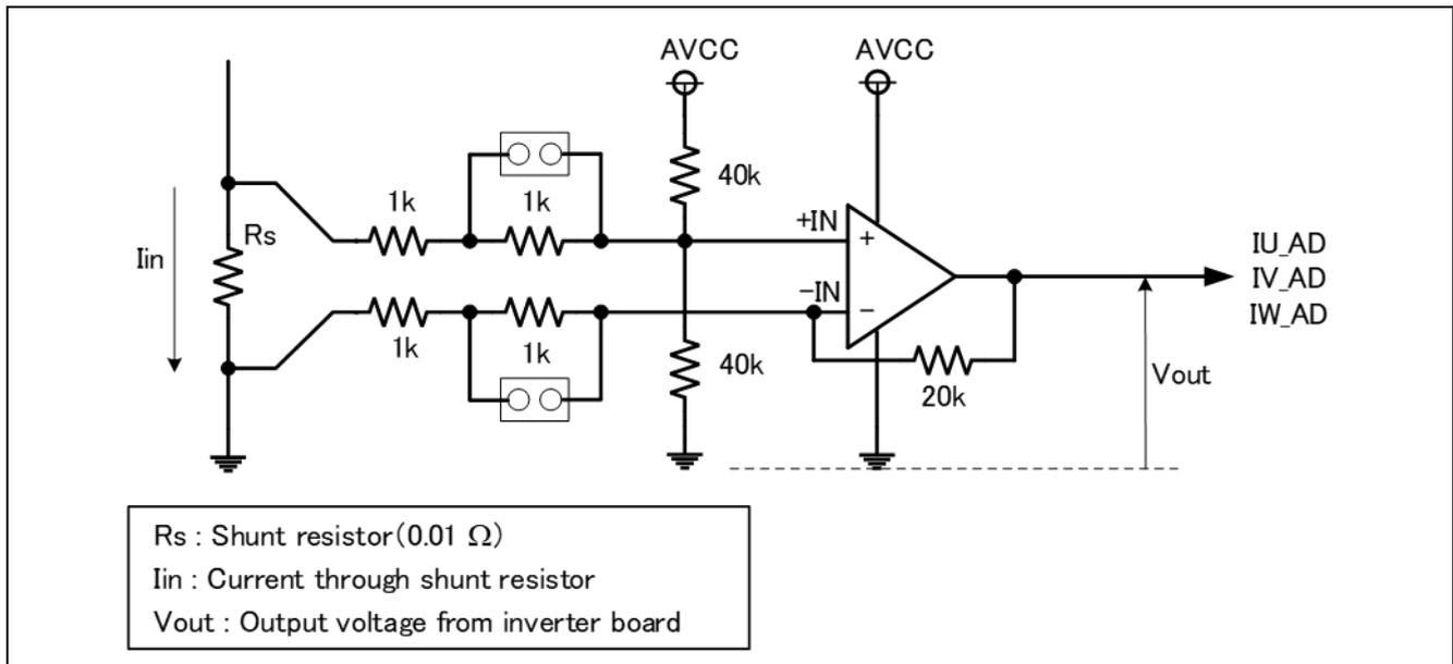
Figure 5-2 Current detection circuit
