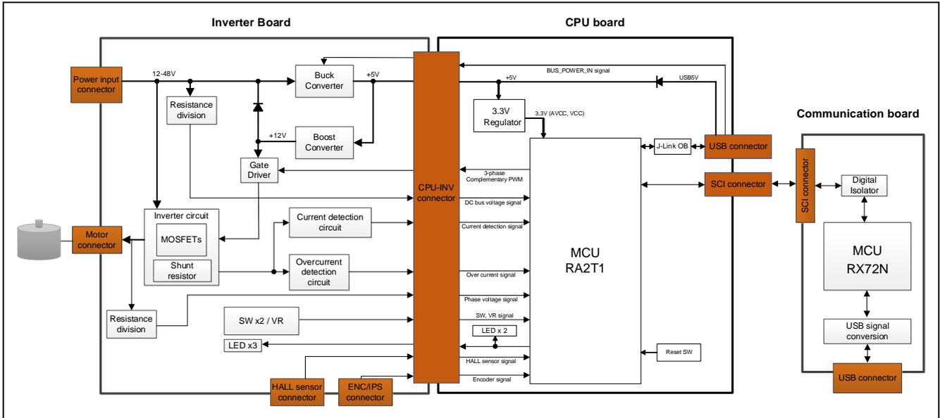
Figure 4-1 MCK-RA2T1 block diagram
