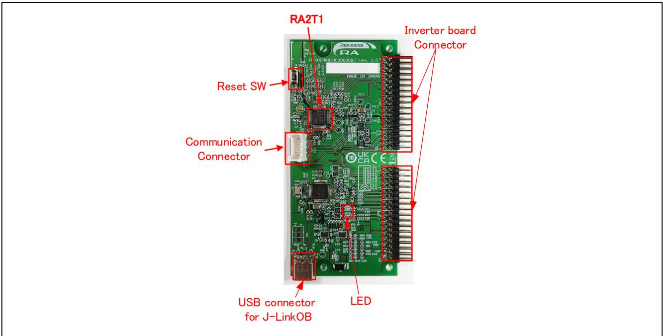
Figure 4-3 CPU Board Layout
