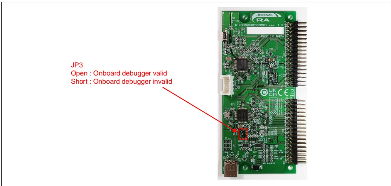
Figure 6-1 Jumper setting of JP3
