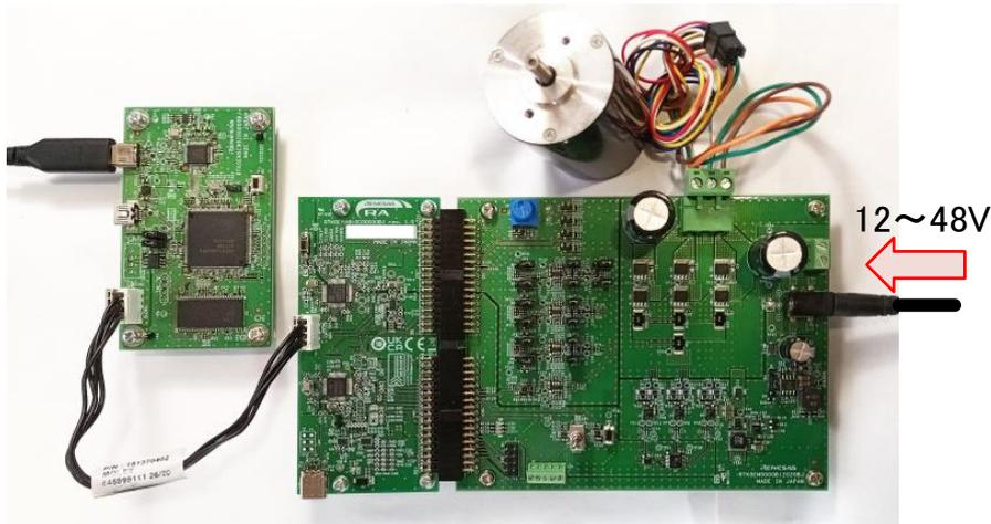
Figure 4-10 Power supply from DC jack
