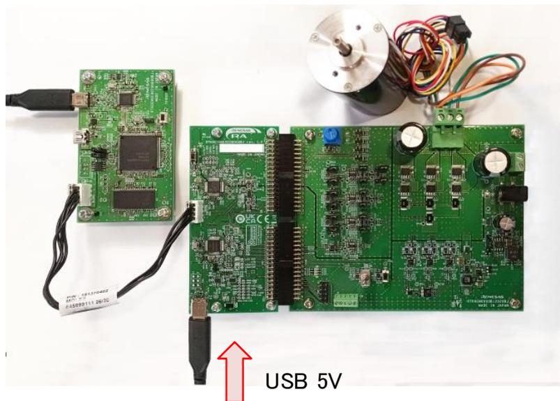
**Figure 4-12 Power supply from USB connector**
