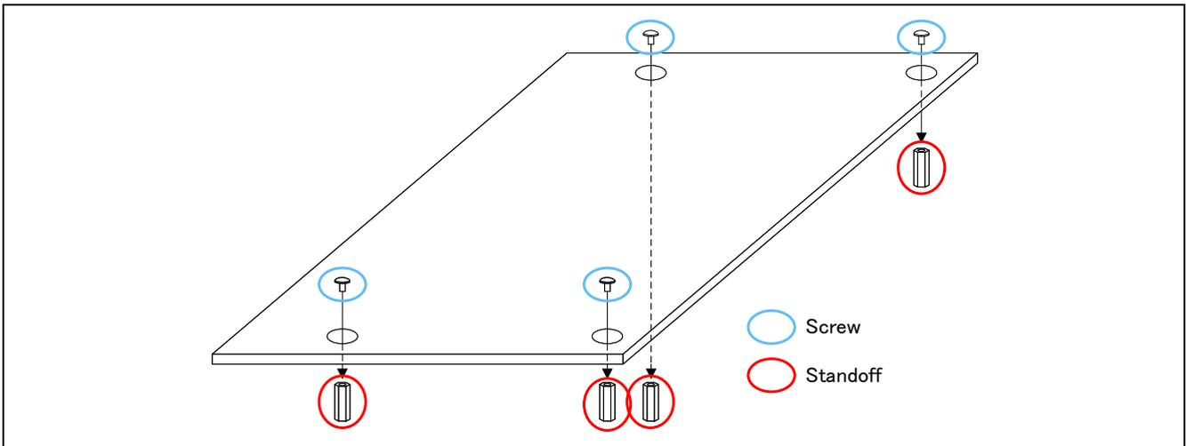
Figure 4-5 Standoffs and Screws assembly
