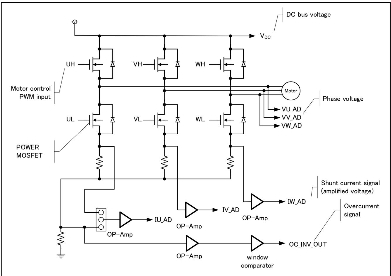
Figure 5-1 Illustration of inverter control circuit block
