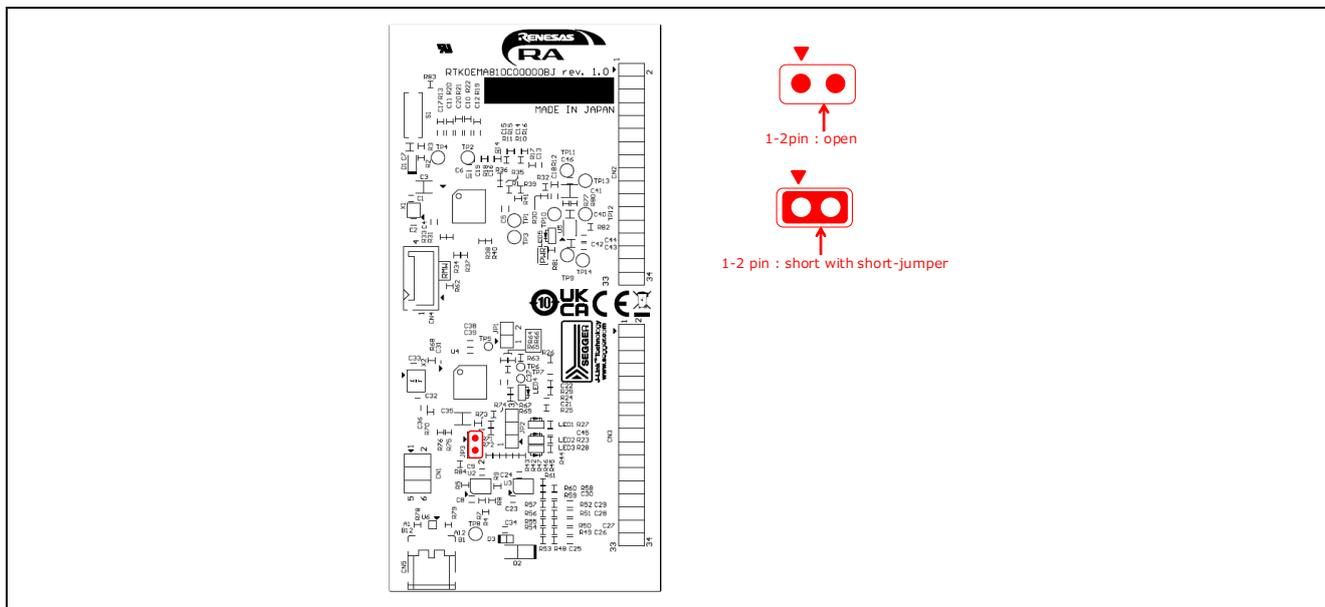
**Figure 4-7 Default jumper pin setting of CPU board**
