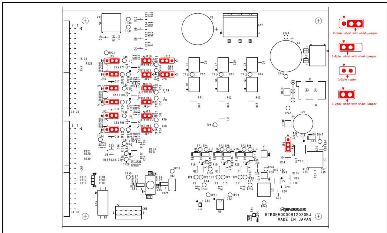
**Figure 4-6 Default jumper pin setting of Inverter board**
