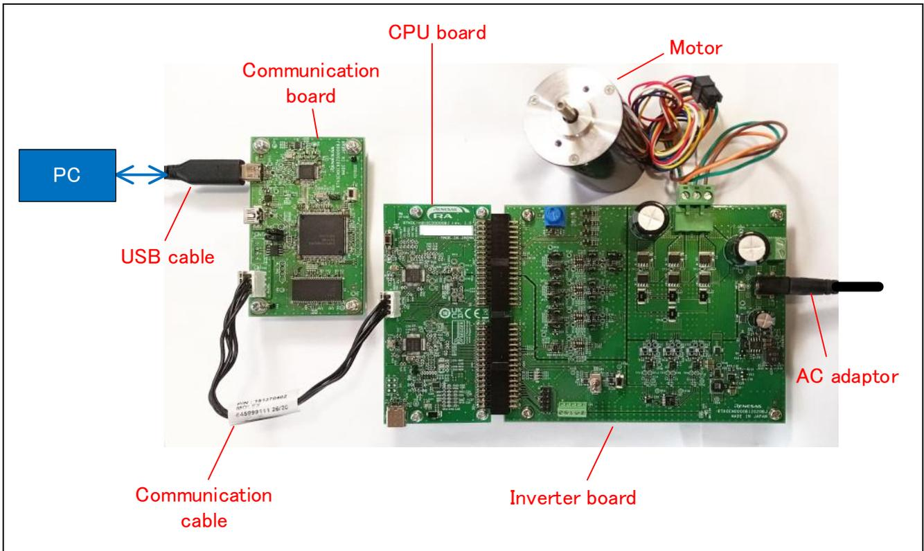
Figure 4-9 Board connection
