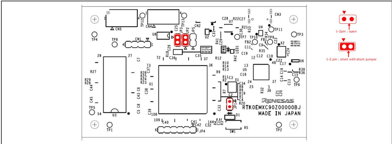
**Figure 4-8 Default jumper pin setting of Communication board**
