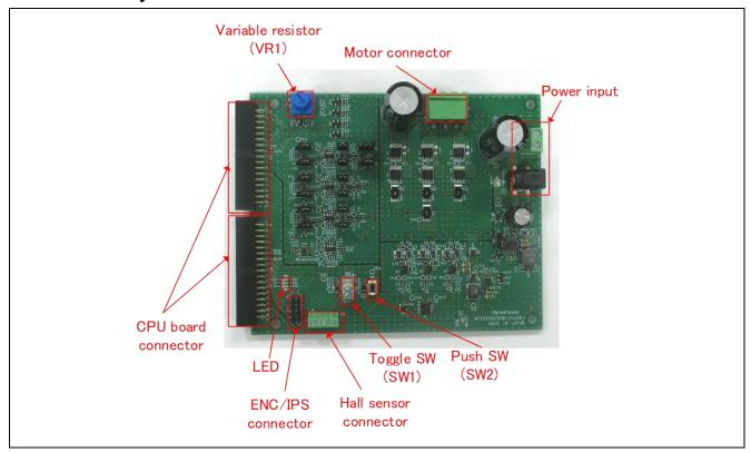
Figure 4-2 Inverter board Layout
