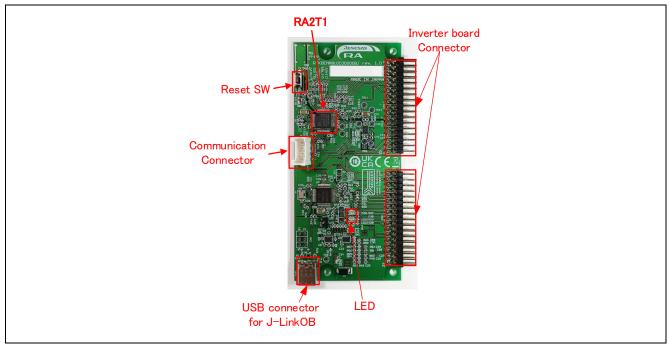
Figure 4-3 CPU Board Layout
