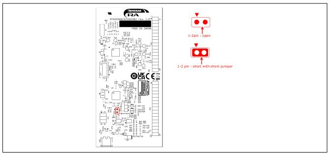
Figure 4-7 Default jumper pin setting of CPU board
