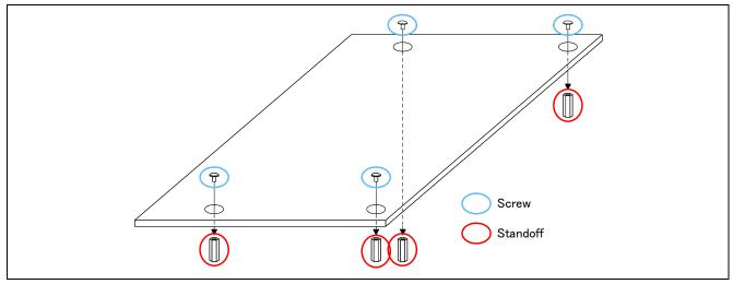
Figure 4-5 Standoffs and Screws assembly
