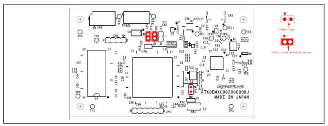
Figure 4-8 Default jumper pin setting of Communication board
