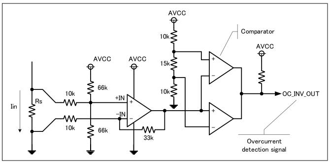
Figure 5-3 Overcurrent detection circuit
