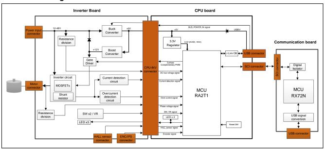
Figure 4-1 MCK-RA2T1 block diagram
