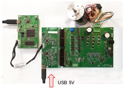
Figure 4-12 Power supply from USB connector
