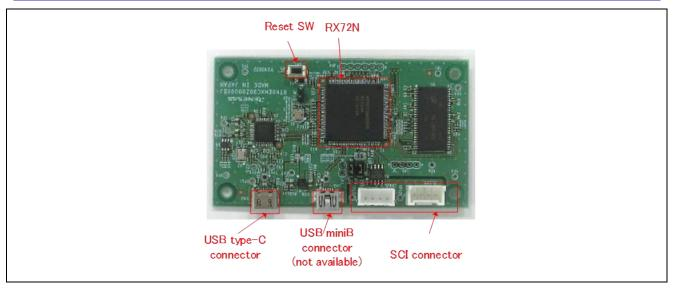
Figure 4-4 Communication board Layout
