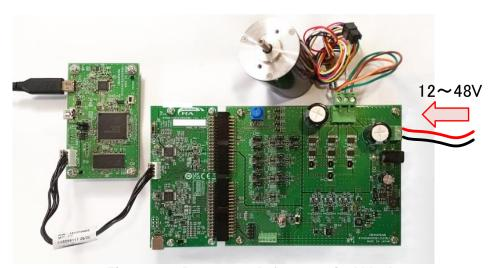
Figure 4-11 Power supply from terminal block
