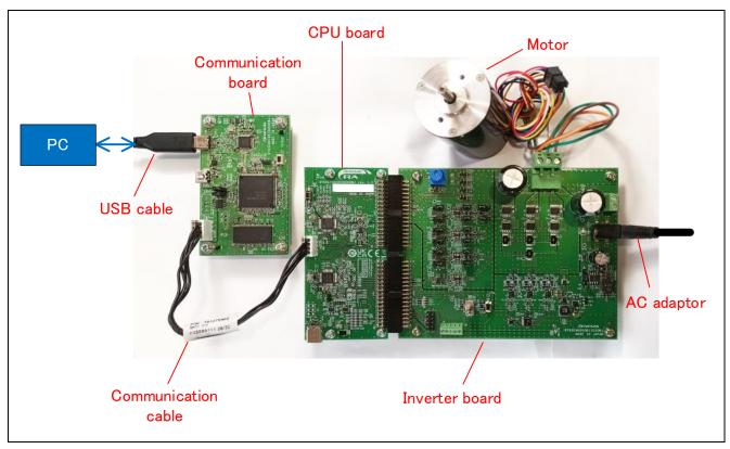
Figure 4-9 Board connection
