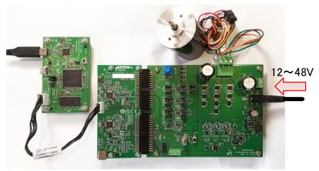
Figure 4-10 Power supply from DC jack
