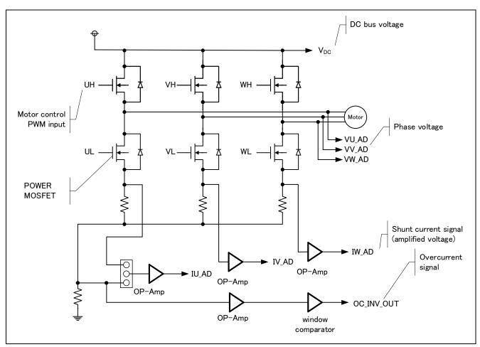
Figure 5-1 Illustration of inverter control circuit block
