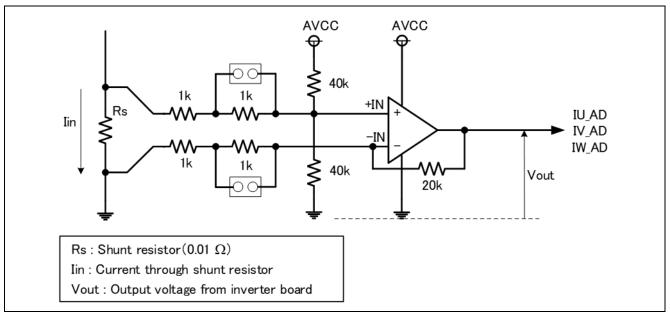
Figure 5-2 Current detection circuit
