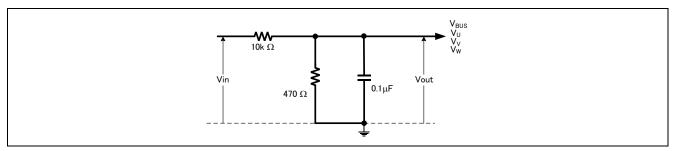
Figure 5-4 Output voltage detection circuit
