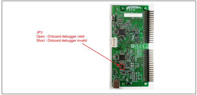
Figure 6-1 Jumper setting of JP3
