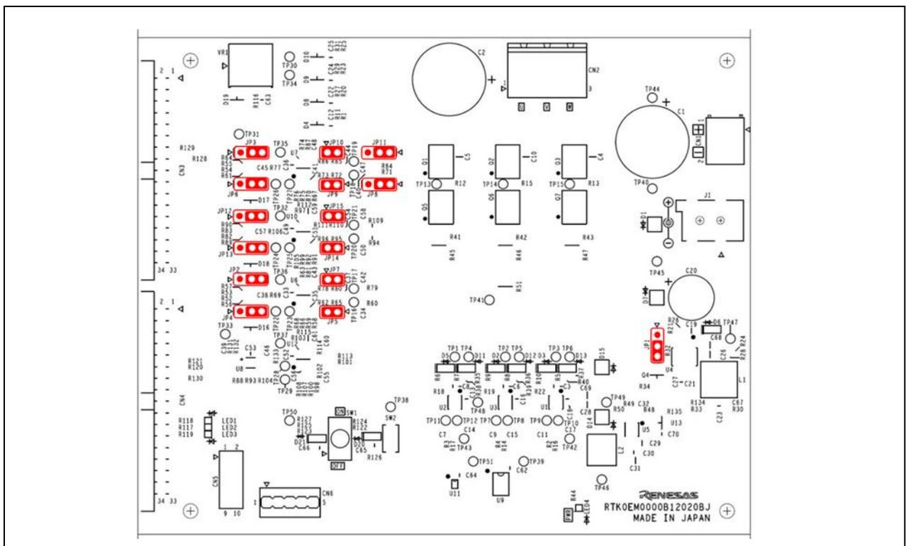
**Figure 4-5 Default jumper pin setting**
