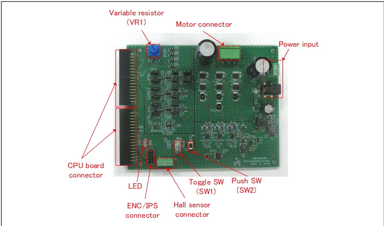
Figure 4-2 Inverter Board
