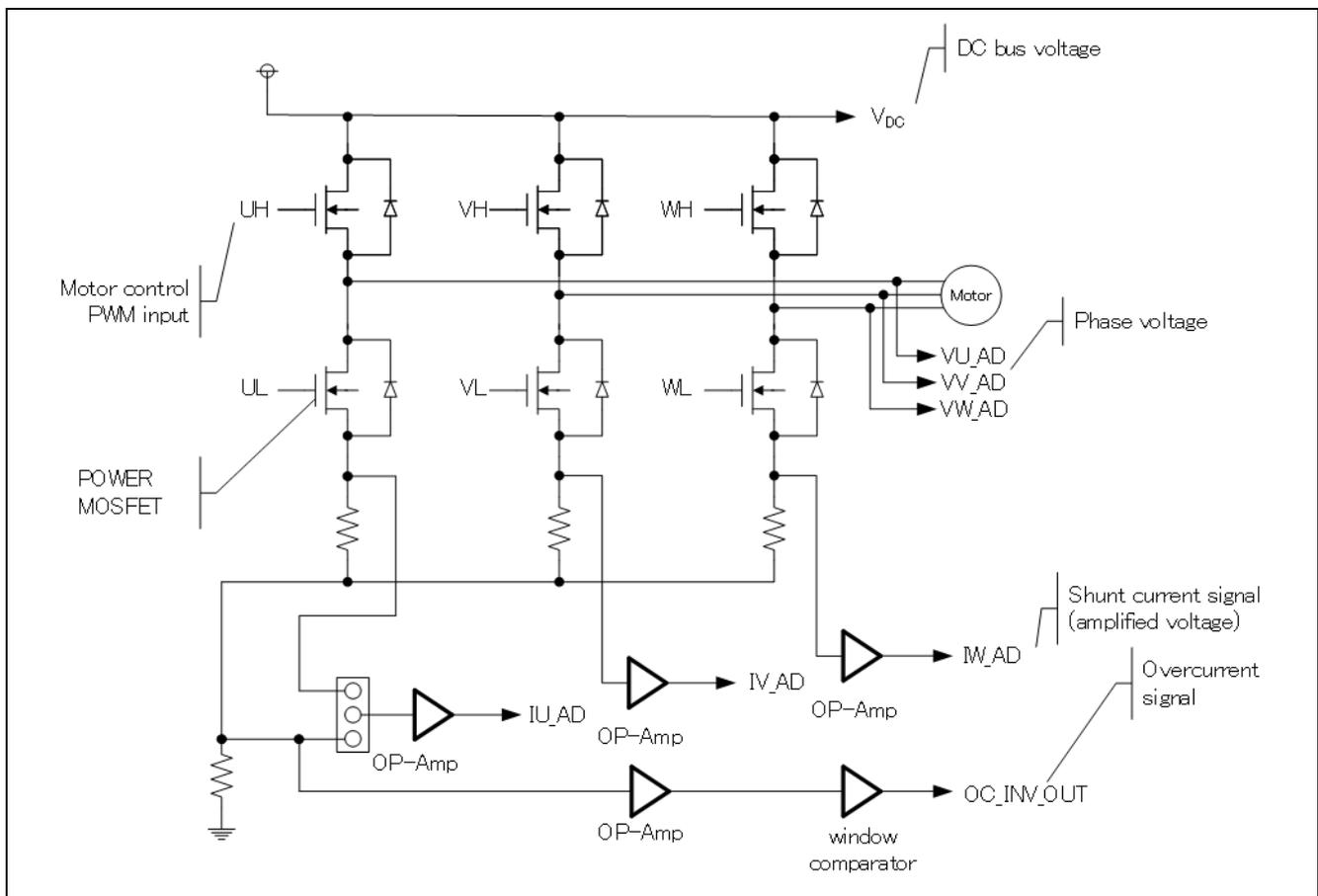
Figure 5-1 Illustration of inverter control circuit block
