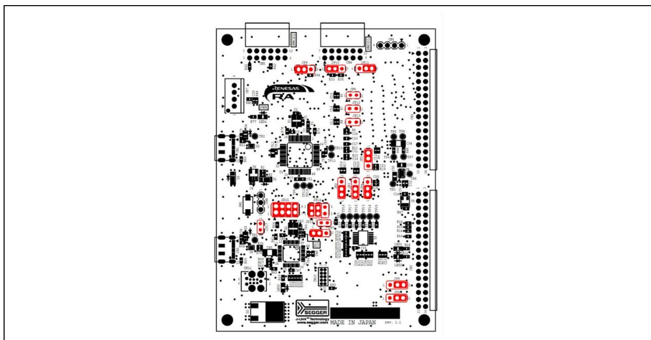
**Figure 4-6 Default jumper pin setting of CPU board**
