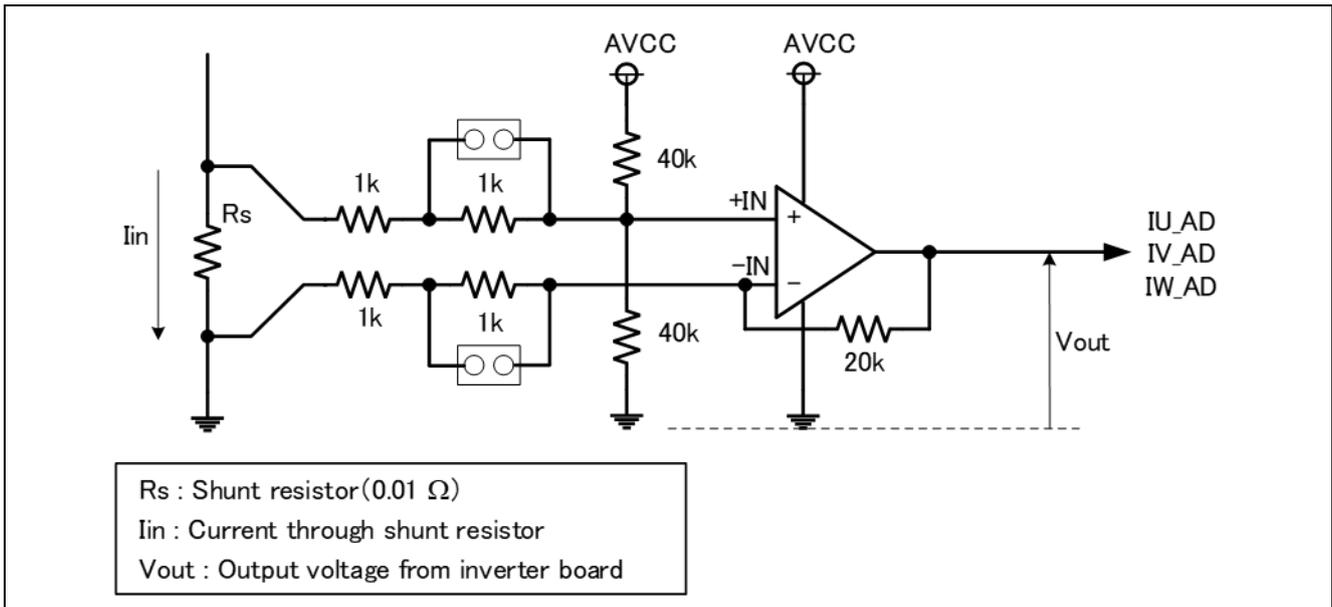
Figure 5-2 Current detection circuit
