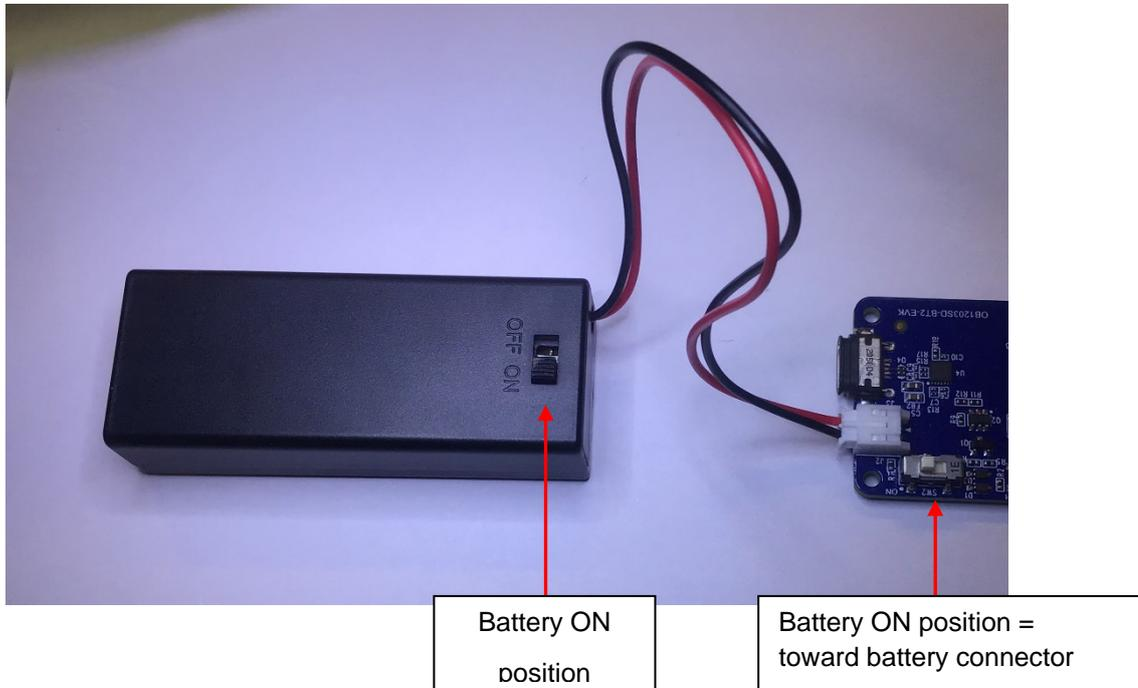
4. Press the push-button switch (SW1) for at least two seconds to wake the EVK electronics. If the battery voltage is above the threshold limit (about 2.2V), the LED next to the switch should turn on solid red indicating that the system is ready for processing sensor measurements.
