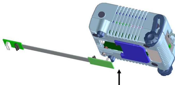
Insert CN1 and CN2 of the probe into TCN1 and TCN2 of the QB-78K0LX3M.
