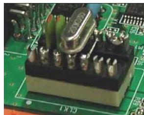
Figure 2-3. Oscillator Shape
