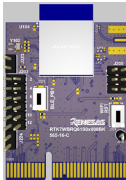
Figure 81. Jumper settings for RRQ61001 daughterboard
