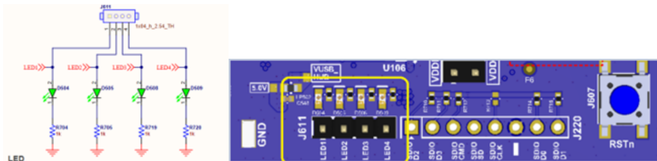
Figure 55. LEDs interface, circuit (left) and PCB locationing
