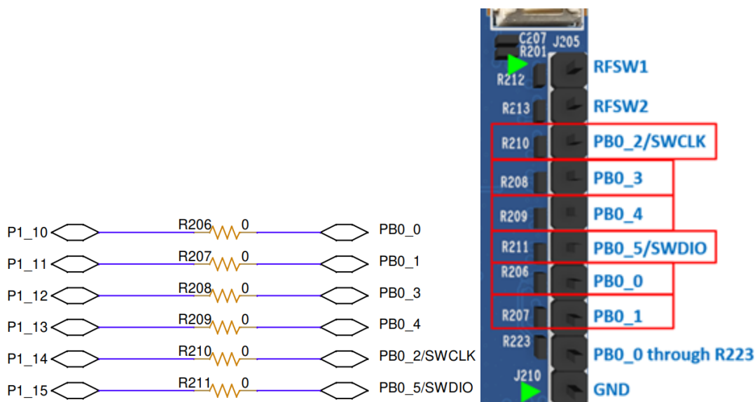
Figure 69. Wi-Fi and Bluetooth LE sections connections on RA6W2 Daughterboard
