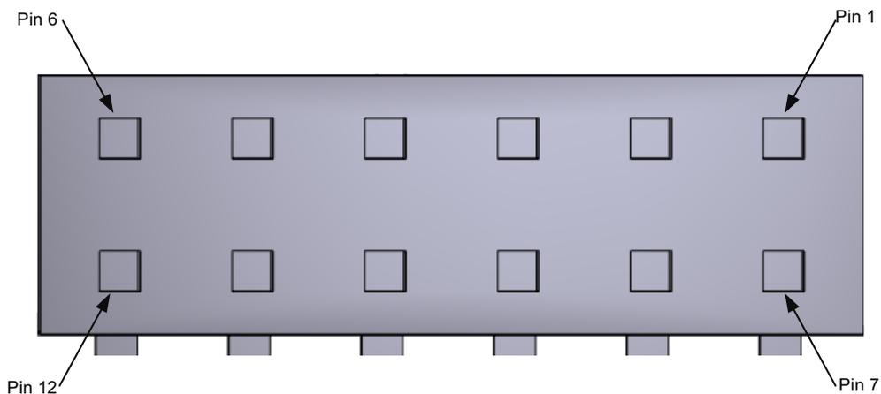
**Figure 5-1: Digilent Pmod™ Compatible Header Pin Numbering**
