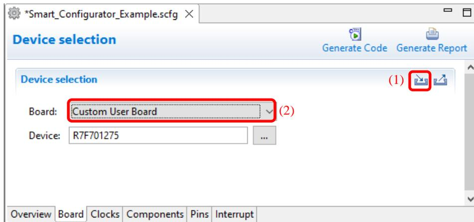
Figure 4-7 Import of Board Configuration (bdf format)
