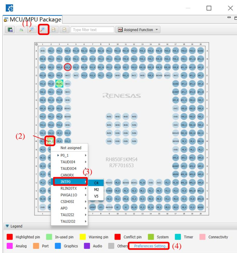
Figure 4-32 Assigning Pins Using the MCU/MPU Package View
