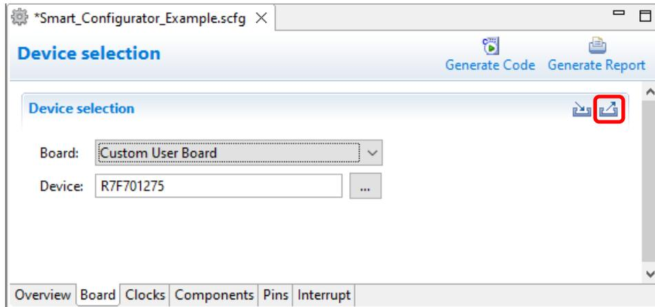
Figure 4-6 Export of Board Configuration (bdf format)
