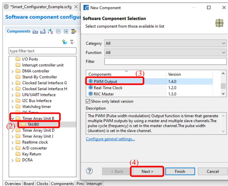
Figure 4-12 Adding CG Components form the Hardware View
