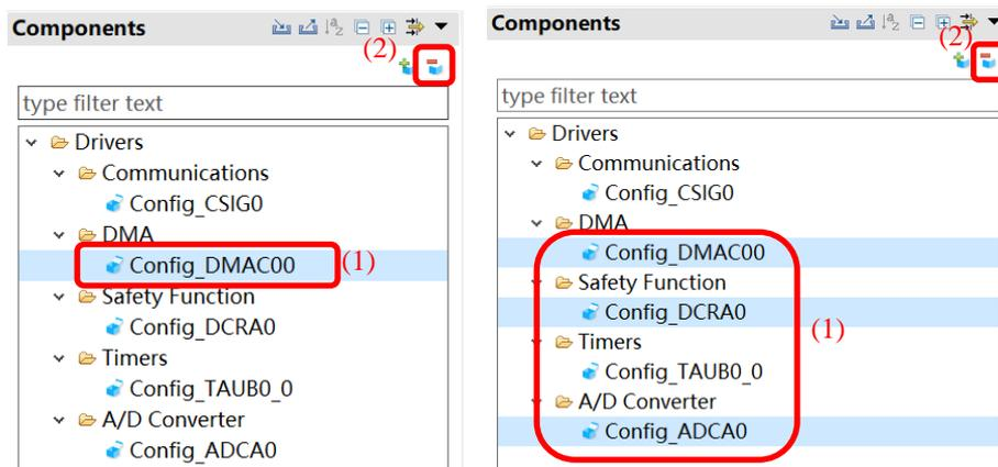
Figure 4-17 Removing a Component or Multiple Components
