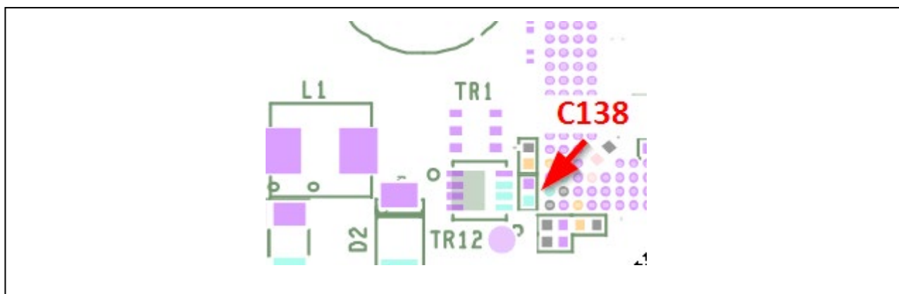
Figure 9.4 Place to add additional capacitors
