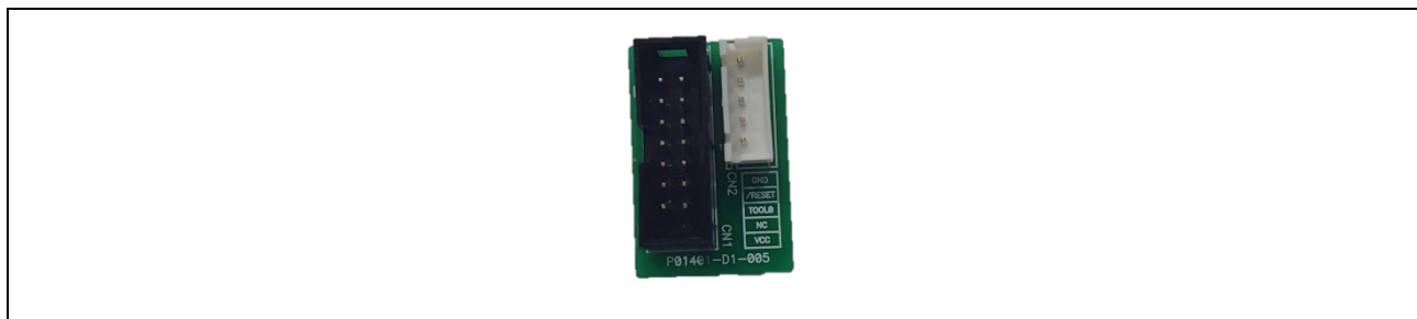
Figure 8-7 Conversion Boards (P014012-1-005)
