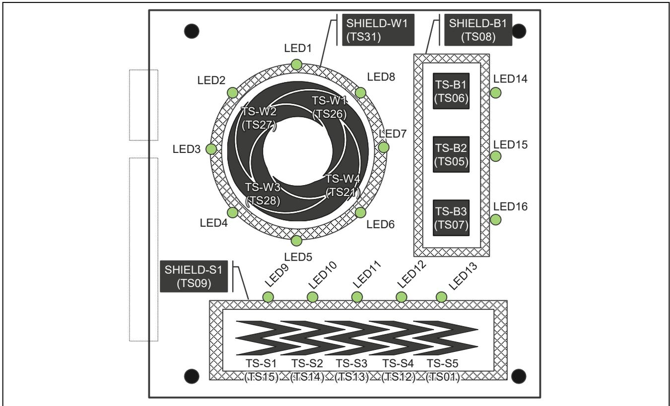
Figure 2. Board Layout and TS Pin Assignments
