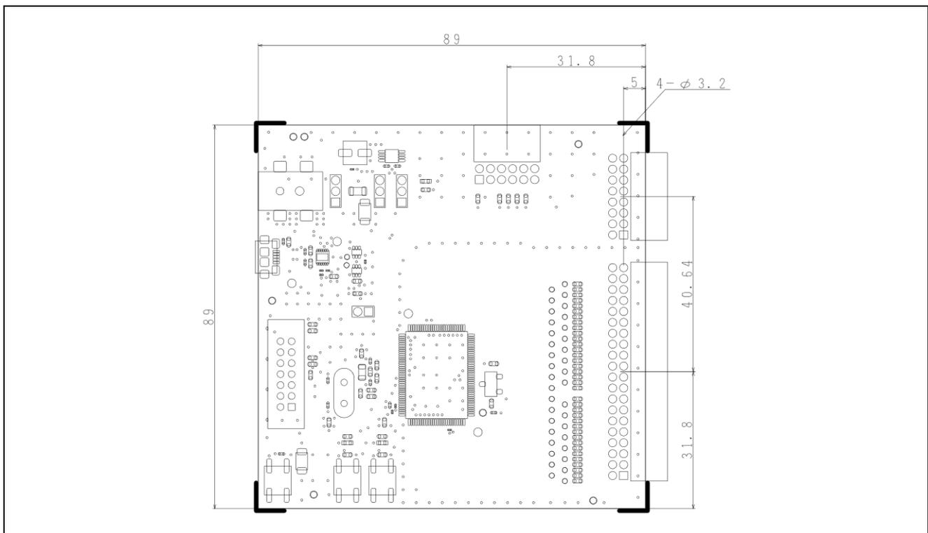
**Figure 2-3. RL78/G23 Cap Touch CPU System Board Dimensions**
