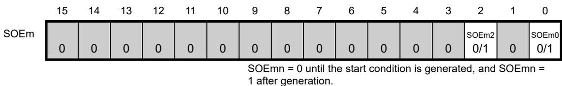
**Note** Only provided for the SCR00 register. This bit is fixed to 1 for the other registers.
