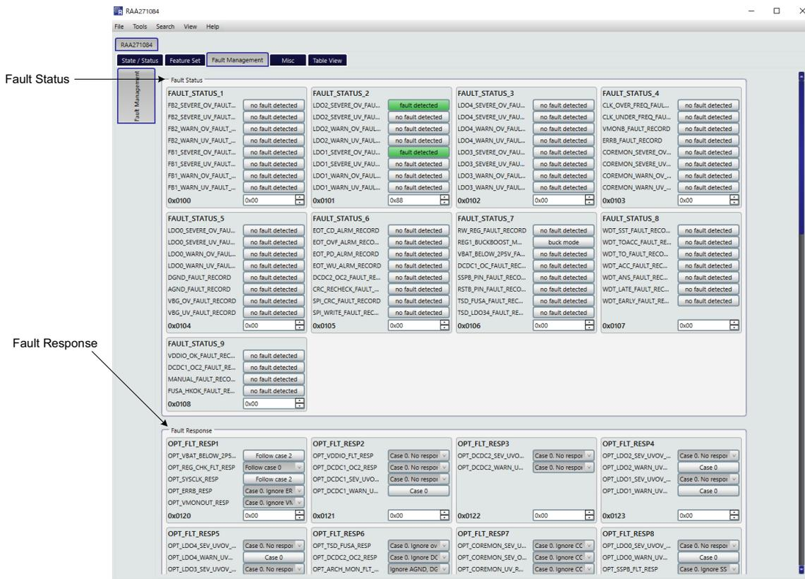
Figure 9. Fault Management (LDO1 and LDO2 Severe OV Detected)
