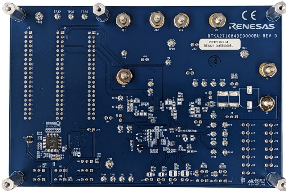
Figure 15. RTKA271084DE0000BU Evaluation Board (Bottom)
