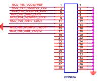
40-pin ribbon cable connector for GPIO/ADC measurements
