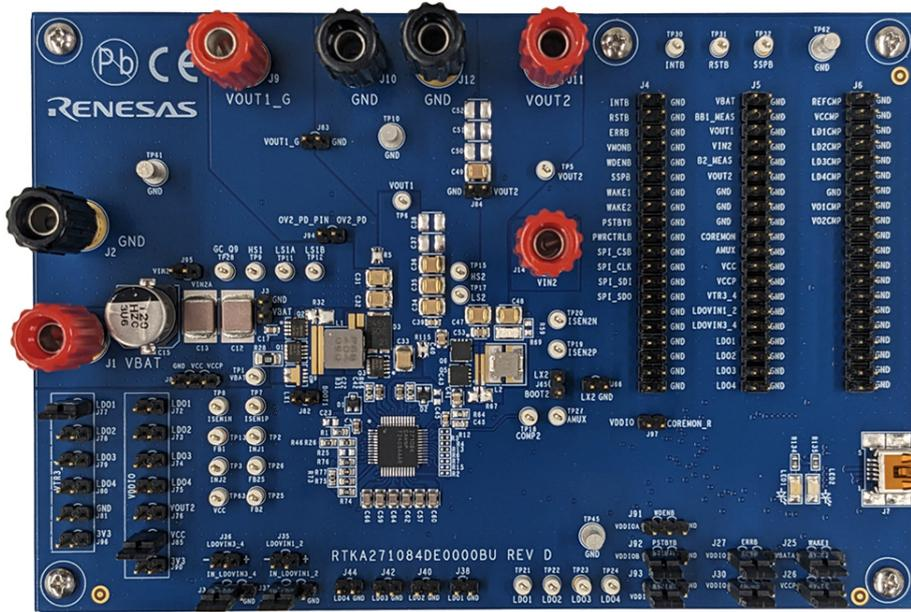
Figure 14. RTKA271084DE0000BU Evaluation Board (Top)
