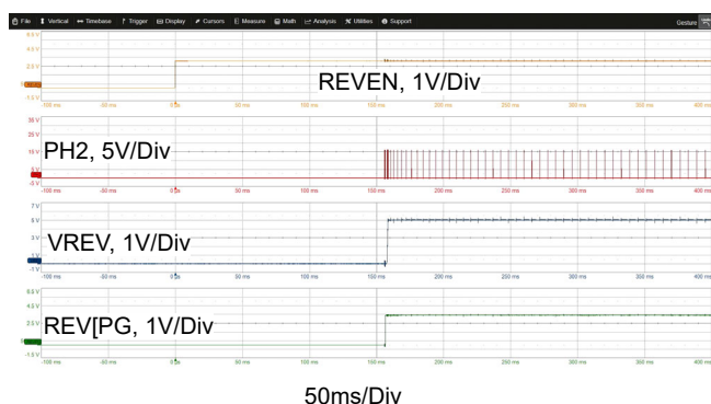
Figure 18. REV Mode Enable, REV_Debounce = 150ms, V_{BAT} = 16V , V_{REV} = 5V
