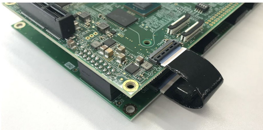
Figure 2.1-2 Connect FFC to RZ/V2N Evaluation Board
