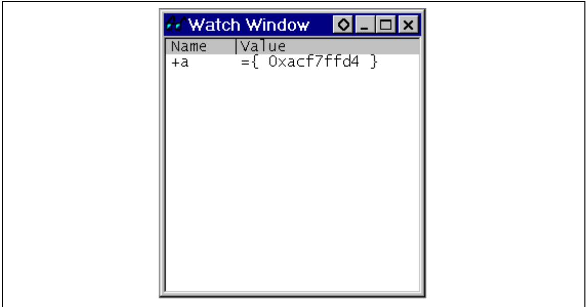
Figure 3.21 [Watch Window] Window (Displaying the Array)
