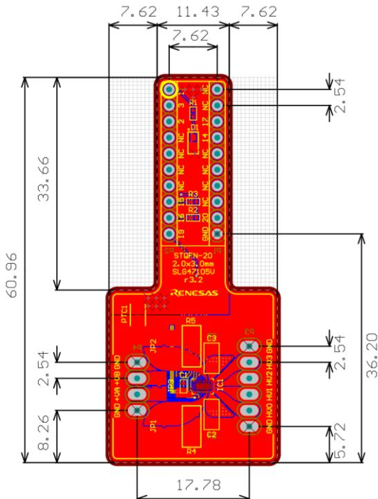
**Note 1** All sizes in millimeters (mm).
