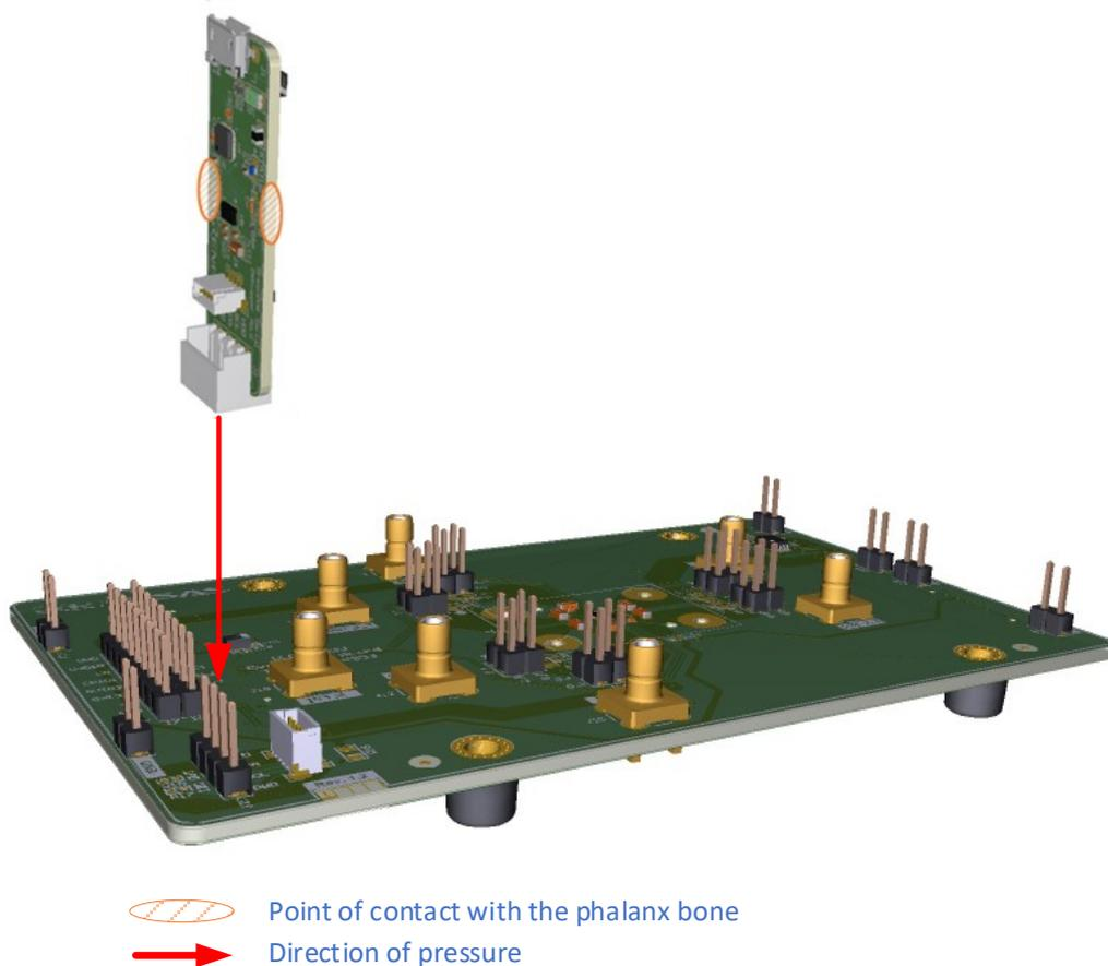
Figure 5. Connecting GSD Board to Evaluation Board
