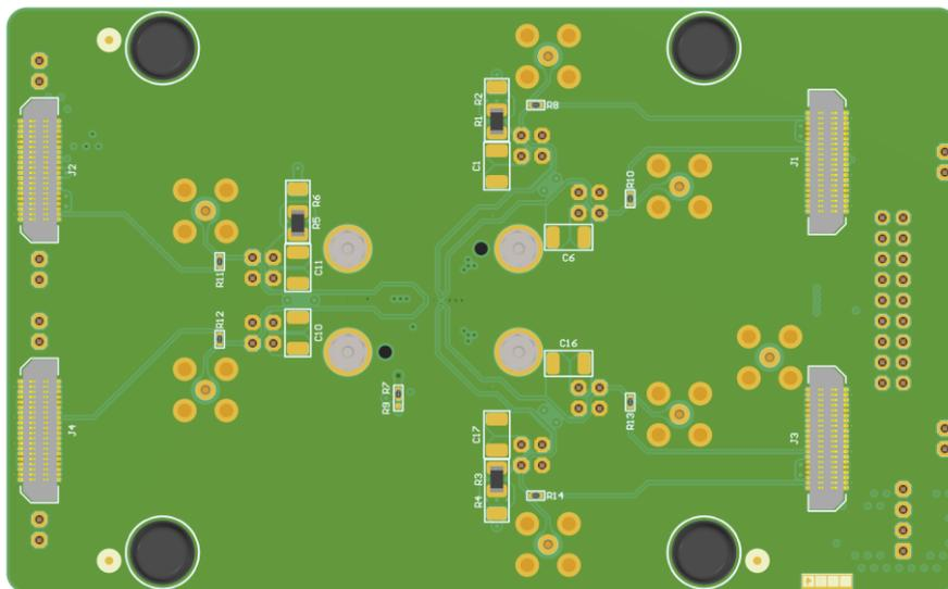
Figure 9. Bottom Side of the Evaluation Board
