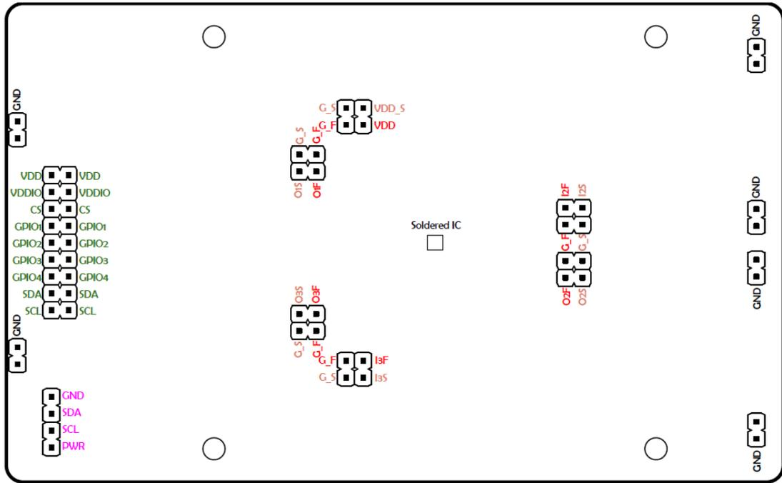
Figure 2. Pin Location of LDO Input/Output with Kelvin Functions Pins, GPIO Pins, GSD Connector on Evaluation Board
