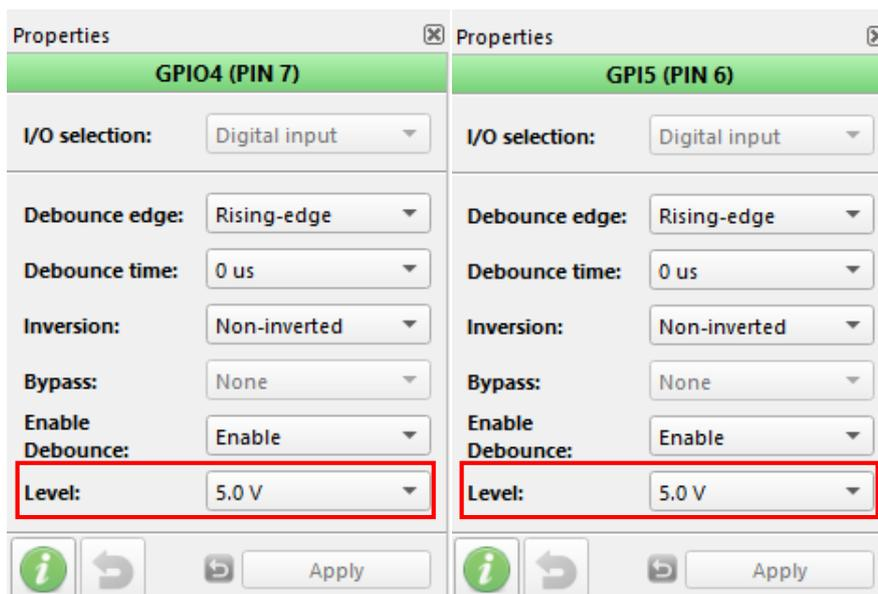
Figure 7. V<sub>DDBUS</sub> Level Settings for I<sup>2</sup>C in Go Configure™ Software Hub
