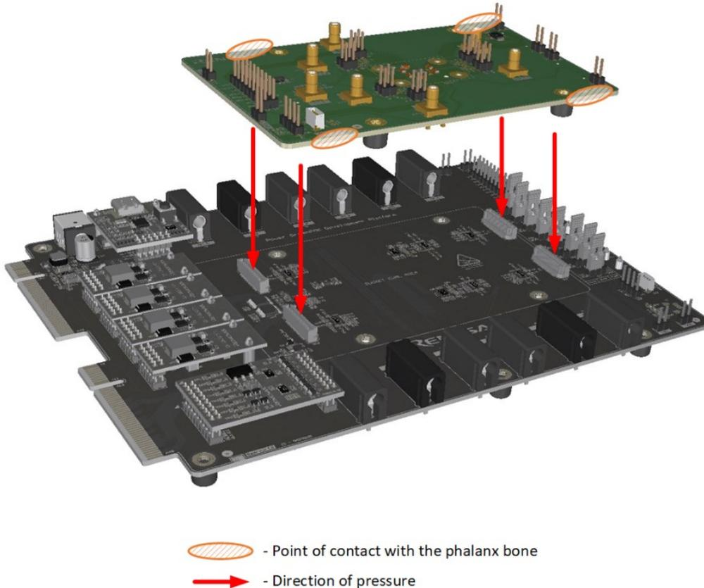
**Figure 10. Inserting Evaluation Board on PGP\_DM**
