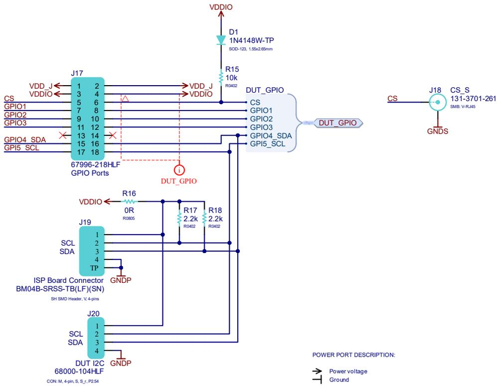
Figure 16. SLG51003V Evaluation Board - GPIO Section Schematic
