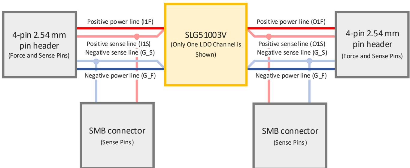
Figure 4. Input/Output Force LDO Pins with Kelvin Functions
