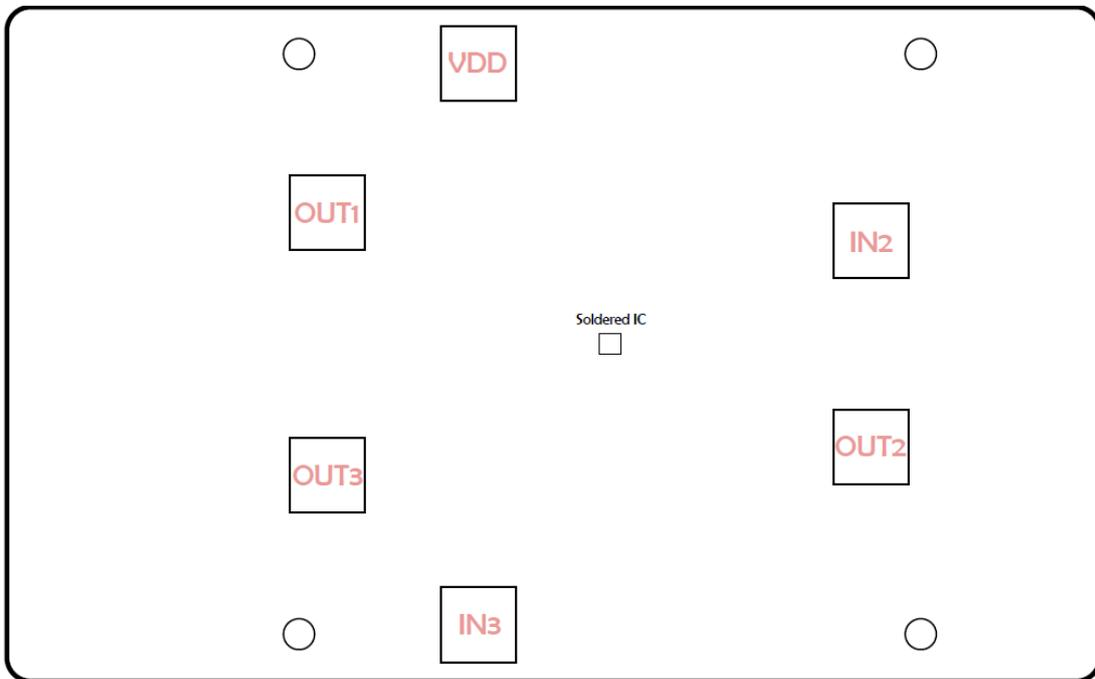
Figure 3. Pin Location of SMB Measurement Connectors on Evaluation Board
