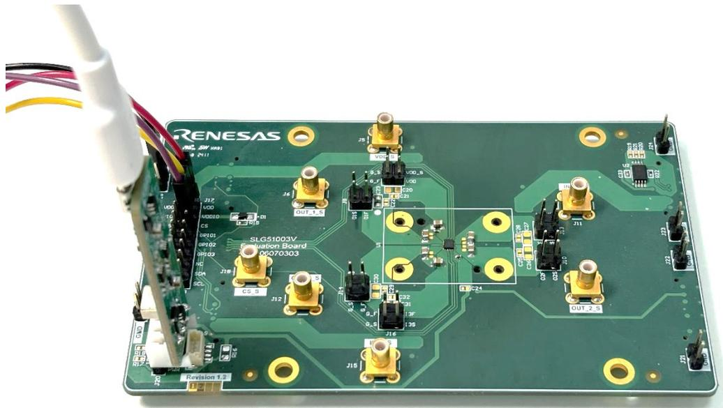
Figure 6. Evaluation Board with GreenPAK Serial Debugger
