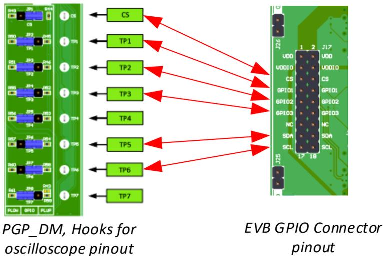
Figure 14. PGP\_DM and SLG51003V-EVB GPIO Connector Pinout Correspondence
