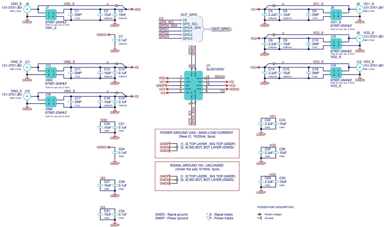
Figure 15. SLG51003V Evaluation Board - Power Section Schematic
