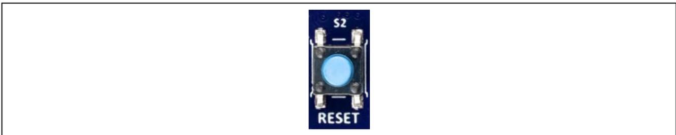
Figure 18. Reset Switch (S2) on Target Board
