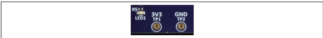
Figure 7. TP1, TP2, and LED1 on Target Board
