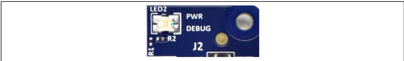
Figure 10. LED2 on Target Board (Top Side)
