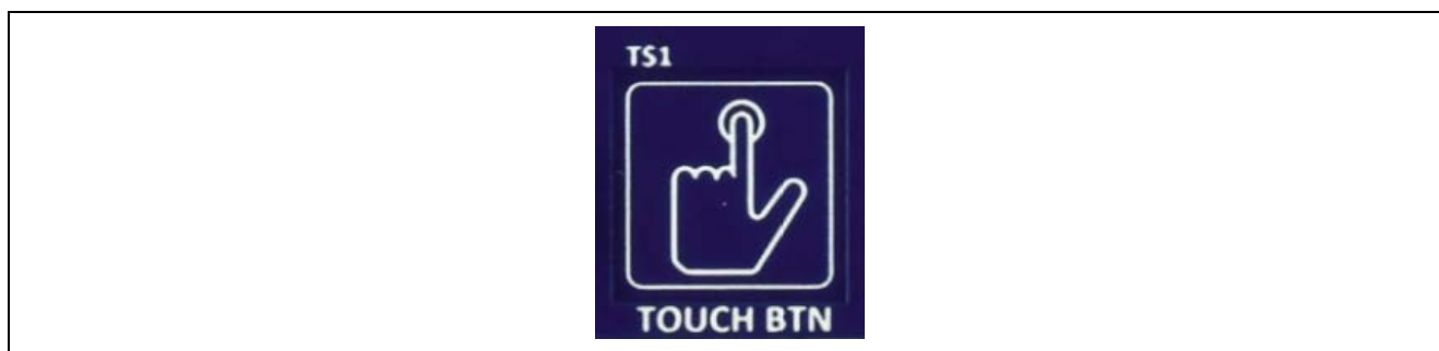
Figure 22. Capacitive Touch Button on the Target Board (Top Side)
