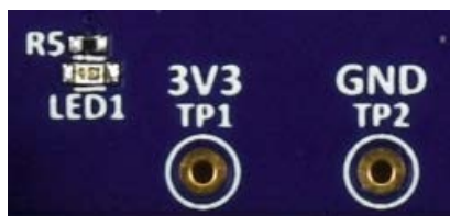
Figure 8. TP1, TP2, and LED1 on the Target Board
