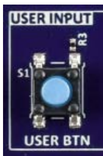
Figure 17. User Switch (S1) on the Target Board
