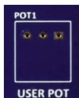
Figure 28. User Potentiometer on the Target Board (Top Side)
