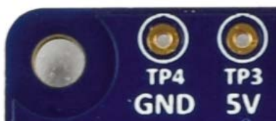
Figure 7. TP3 and TP4 on the Target Board
