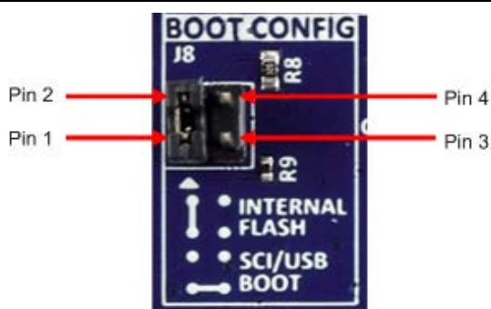
Figure 29. Boot Config Jumper J8
