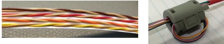
Figure 123: Example of Twisted Pair Cable with 4 Pairs and Ferrite
